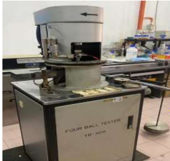
Figure 3.7: Four ball tester in Tribology Lab University Malaya
