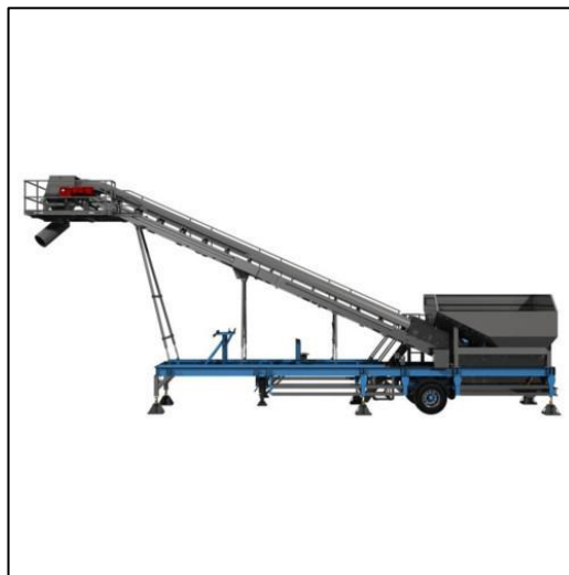
Mobile Conveyor Belt to be installed on the track system
