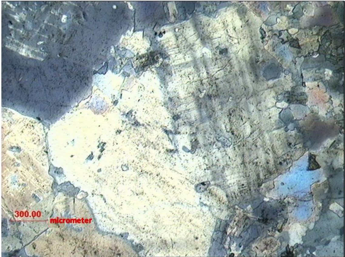
Figure 3.8c.: Photomicrograph of sample UM/GLG/2005/C. The quartz and microcline porphyroblasts are seen as individual grains.
