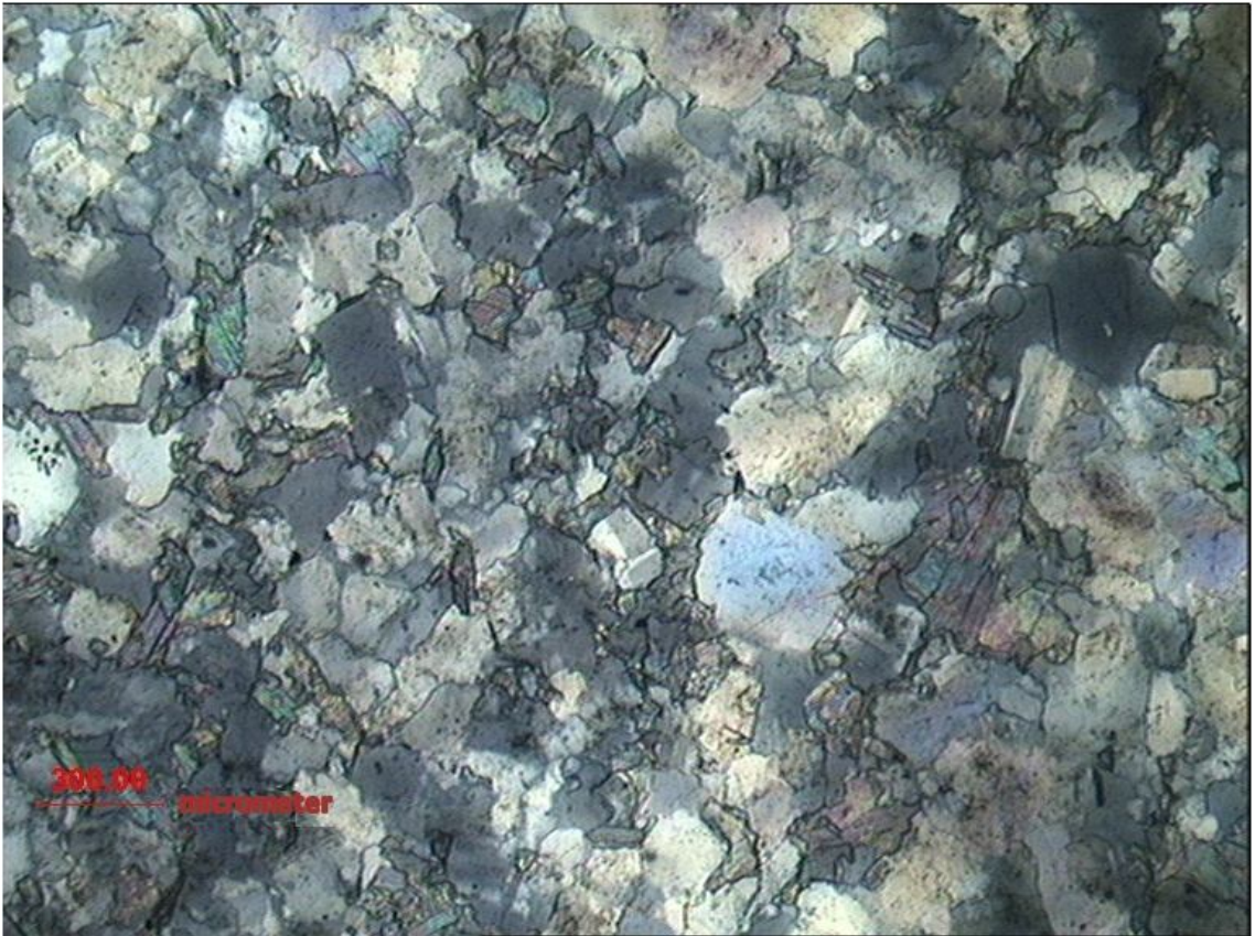
Figure 3.8a.: Granite photomicrograph of sample UM/GLG/2005/C. The quartz is translucent with flecks of muscovite, biotite, and k-feldspars. Magnification. : 2.5x. (Scale in left-hand corner is 0.3 mm long).
