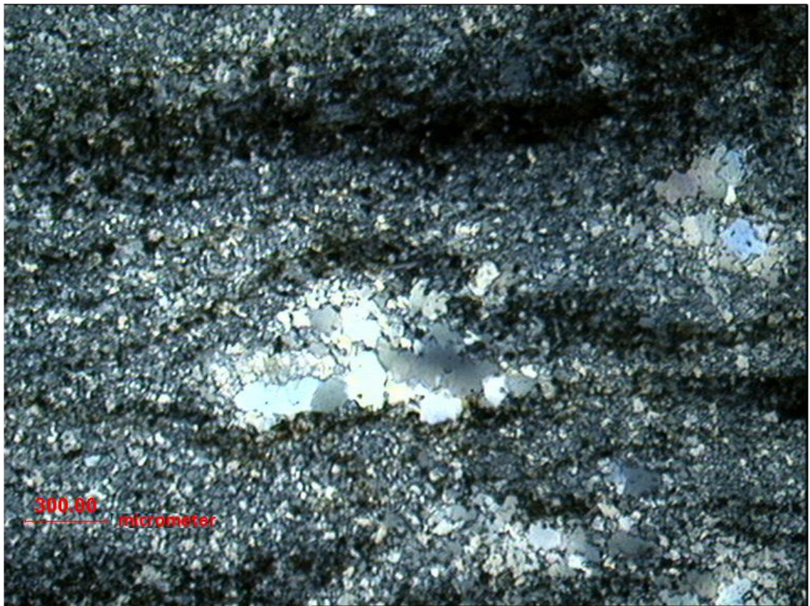
Figure 3.6a.: Photomicrograph of sample UM/GLG/2005/A showing irregular quartz porphyroblasts in fine grained matrix of quartz and muscovite. Magnification.: 2.5x (Scale in left-hand corner is 0.3 mm long).
