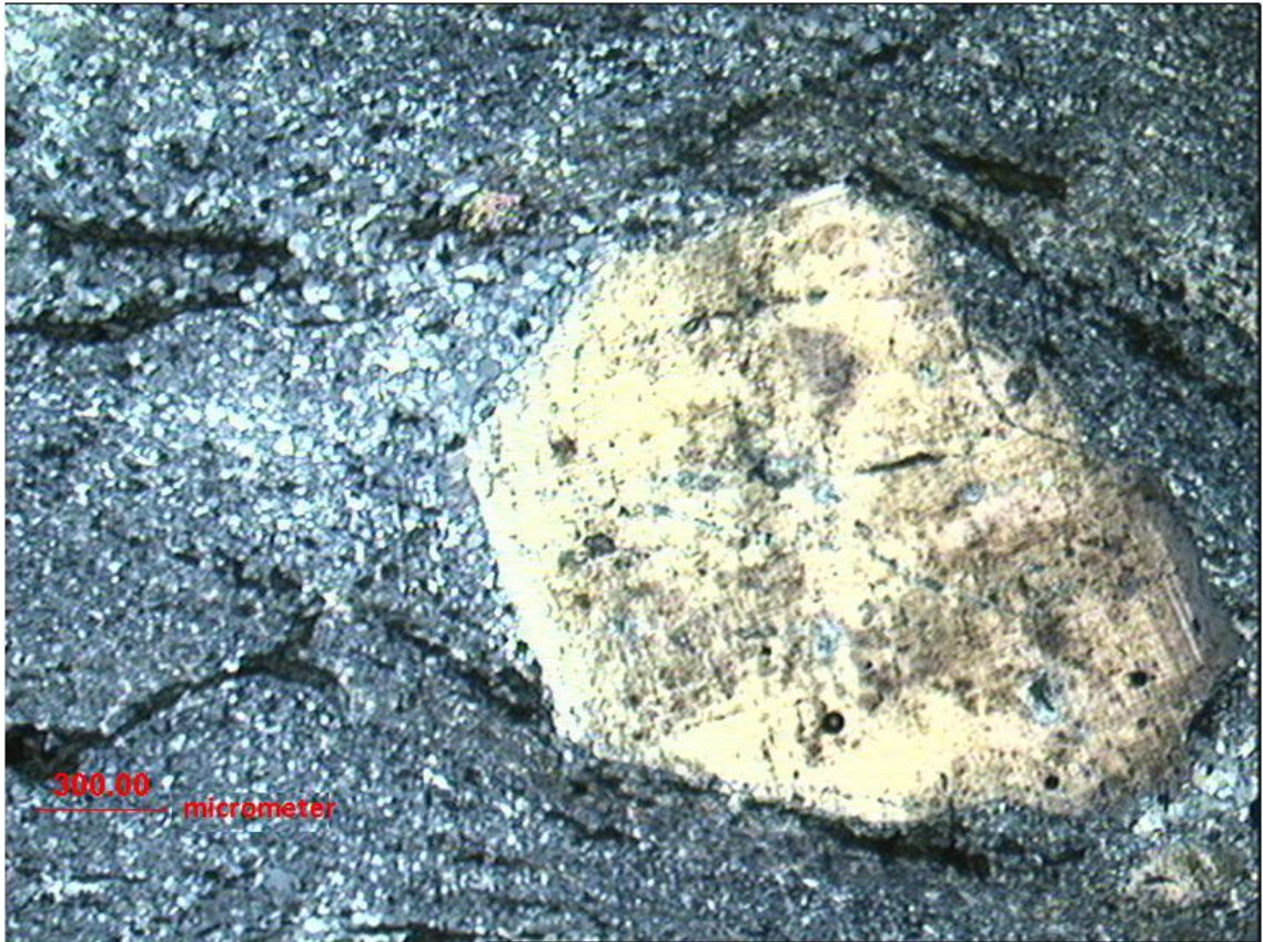
Figure 3.6b.: Photomicrograph of sample UM/GLG/2005/A showing relic microcline within matrix of fine grained quartz and muscovite.
