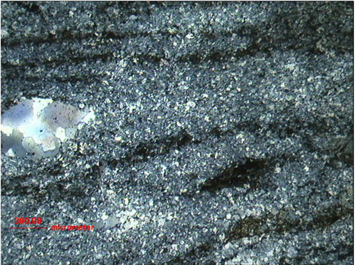
Figure 3.7a.: Photomicrograph of sample UM/GLG/2005/B showing quartz porphyroblast within an aligned matrix of fine grained quartz , muscovite and biotite. Magnification.: 2.5x. (Scale in left-hand corner is 0.3 mm long).
