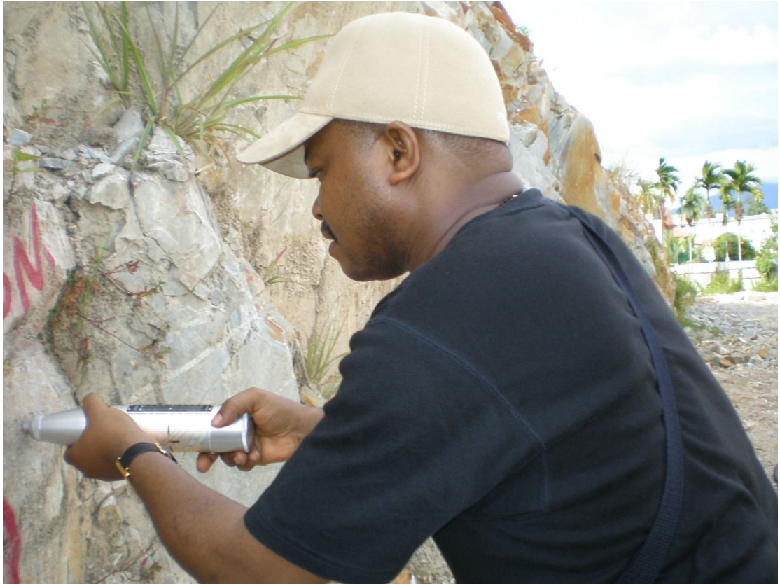
Fig. 4.9. The writer using the Schmidt hammer model N on in-situ rocks in Taman Ukay Perdana.
