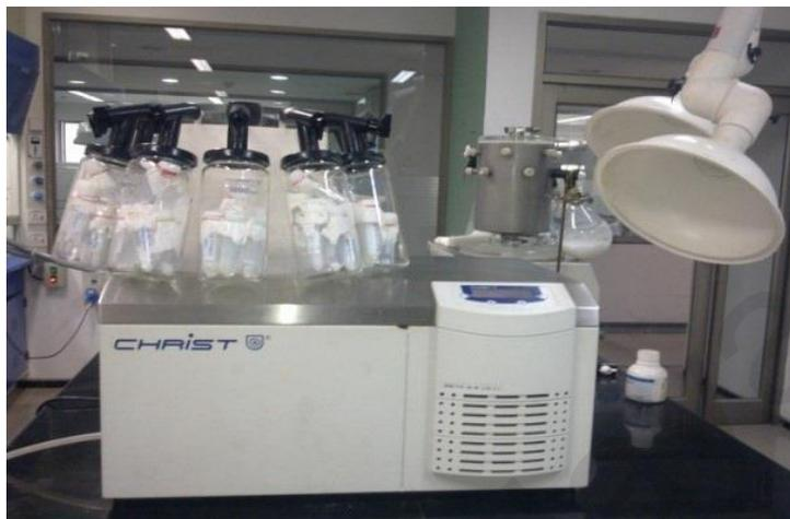
**Figure 4.22: Freeze dryer used in this study for lyophilisation process.**
