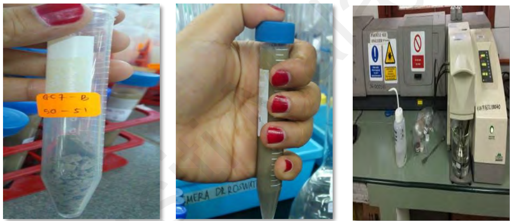
Figure 3.3: Preparations of sediment samples for particle size analysis using Malvern Mastersizer.
