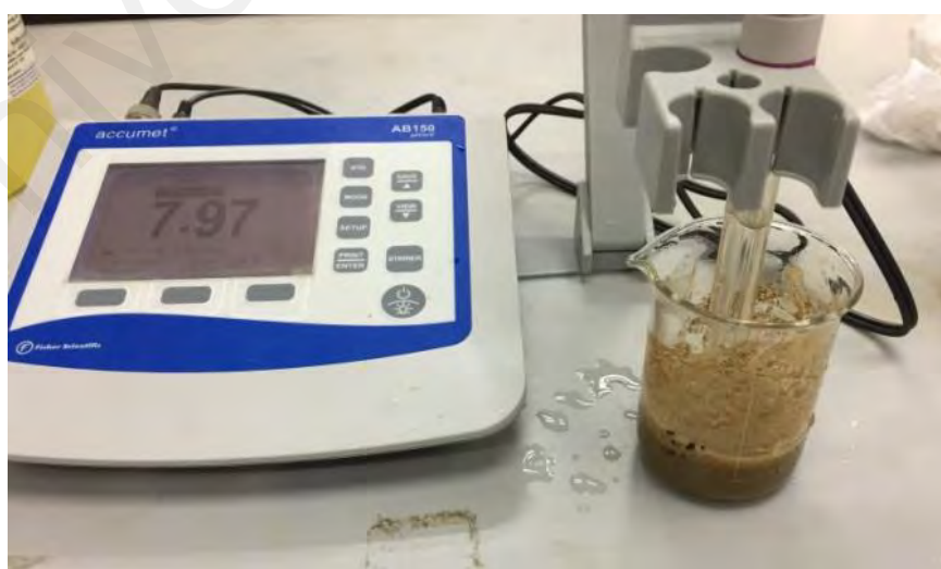
Figure 3.4: Image showing sediment being analysed with digital electrode pH meter (Model WTW ph 330).
