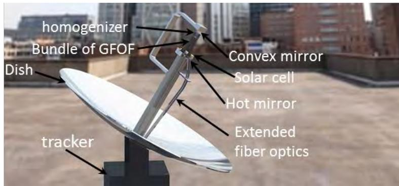
**Figure 6-19: CAD prototype of the system**
