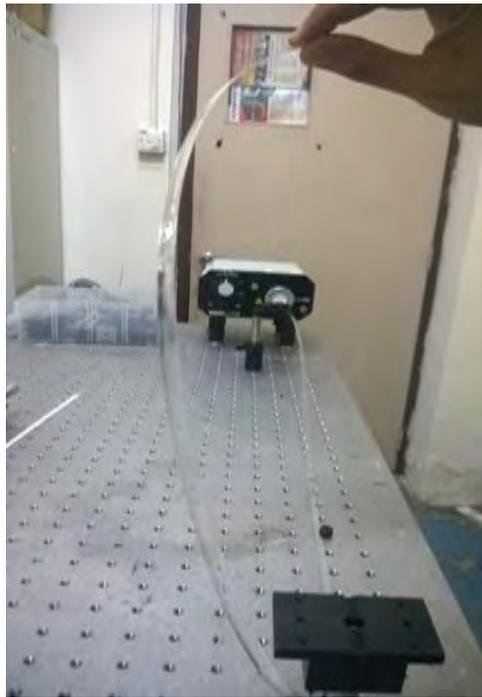
**Figure 5-20: flexibility of flat fiber in bending and twisting**
