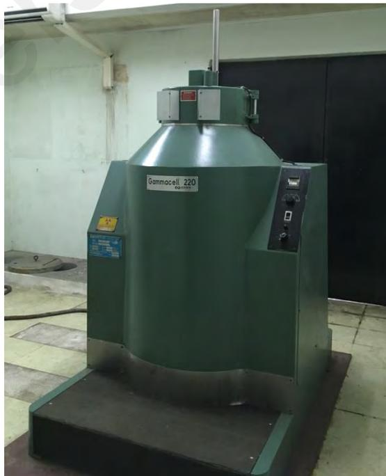
**Figure 3.2:** Gammacell 220 at Physics Laboratory used to irradiate the plantlets.
