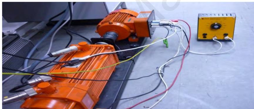
**Figure 4.23: Laboratory procedure for assessing the open-circuit fault in the stator, with wavelet index**
