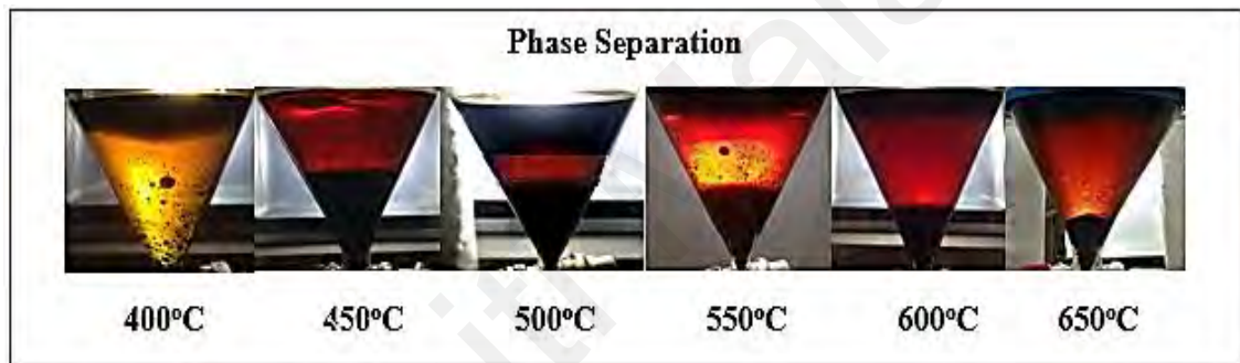
Figure 4. 12: Phase separation of bio-oil with various temperatures under the influence of gravity.
