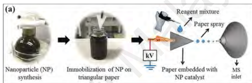
Figure 4.8: Schematic illustration of the nanocatalyst-embedded paper for the reactive paper spray methods (Banerjee et al., 2016).
