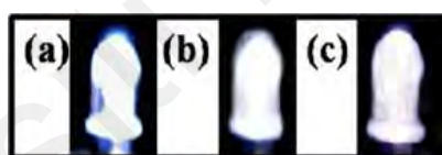
Figure 2.13: Photographs of commercially available UV-LED coated with white light emitting solutions: (a) D1-A1 (b) D2-A1 (c) D2-A2 (Maiti et al., 2013).
