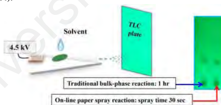
Figure 4.6: Online paper spray reaction (from spotted starting reagents) collected on a TLC plate (left); Chromatographic separation on TLC plate (right) (Bain et al., 2014).
