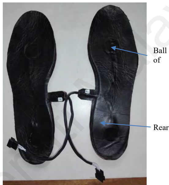
Figure 6.3: Insole ground reaction force sensor
