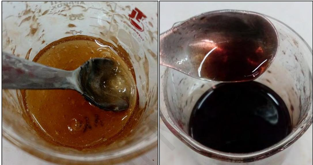
**Figure 4.2: Dissolution of CFF in BMIMCl at 110 °C; before (left) and after (right)**
