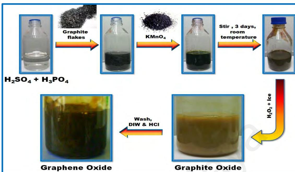
**Figure 3.1.** Schematic representation for the synthesis of GO using simplified Hummers' method.
