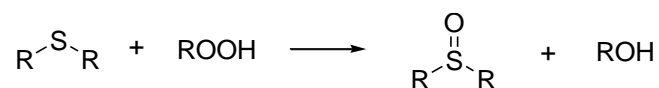
Figure 2.7: General reaction between dialkyl sulfides with hydroperoxide molecules by converting them to sulfoxides (Soleimani et al., 2018)
