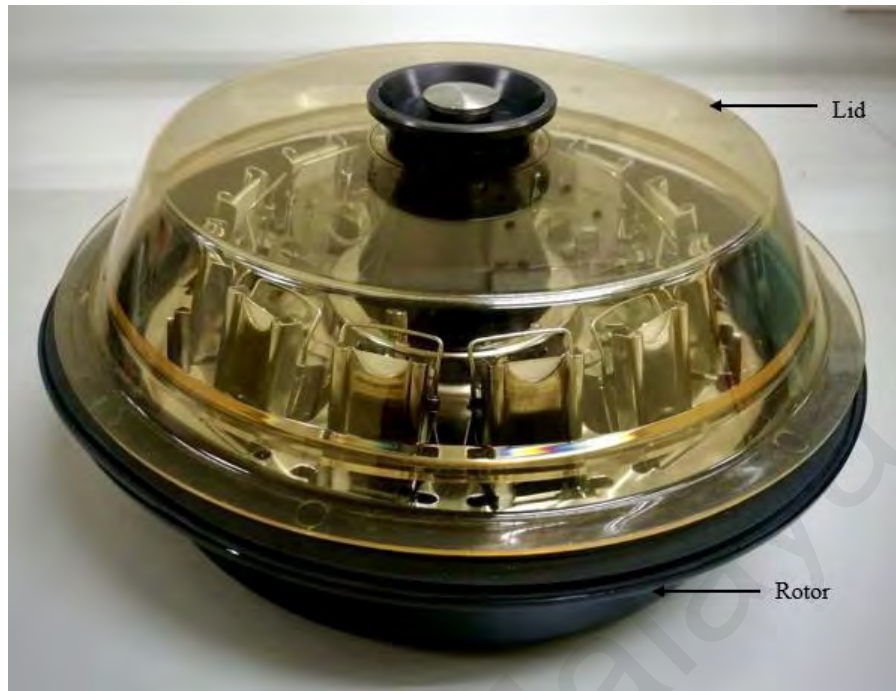
Figure 3. 3: Assembled cytology funnels on the metal stages arranged on the sealed rotor.
