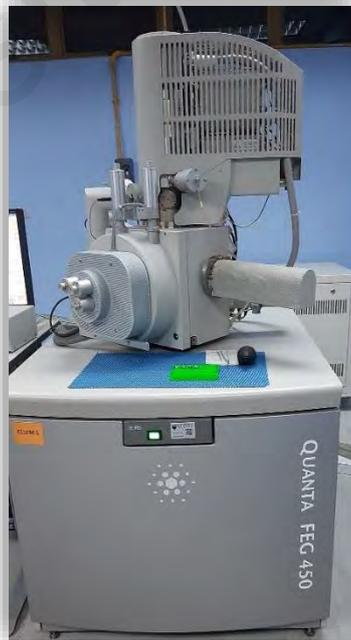
**Figure 3.5:** An image of the Quanta FEC 450 FESEM equipment.
