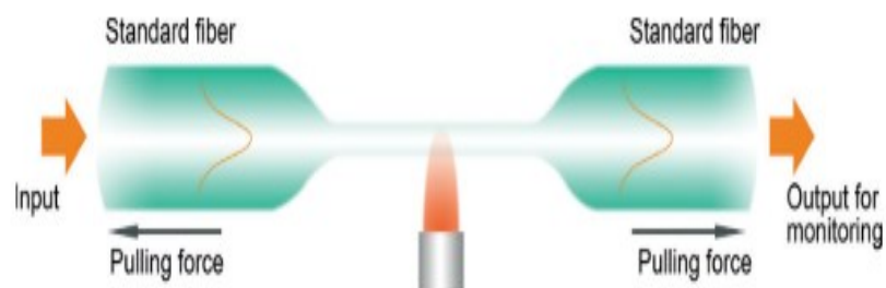
Figure 2.9: Fabrication technique of the microfiber using flame heated source (Wu & Tong, 2013)
