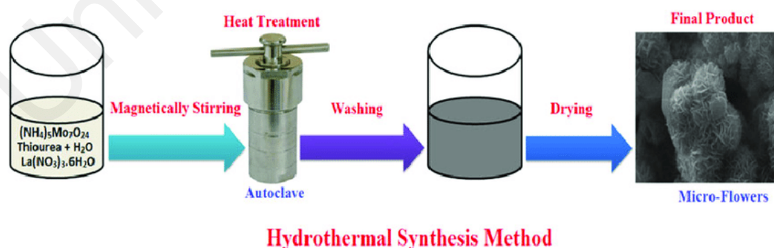
Figure 2.5: Hydrothermal synthesis process for 3D flower-like MoS 2 nanostructure (Nadeem Riaz et al., 2019)
