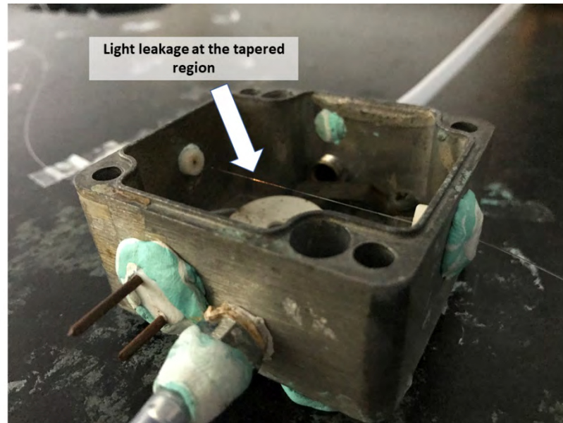
Figure 3.16: Light propagates into the tapered optical fiber sensor.
