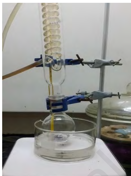
Figure 3.8: Oxidation reaction (catalysis) setup.
