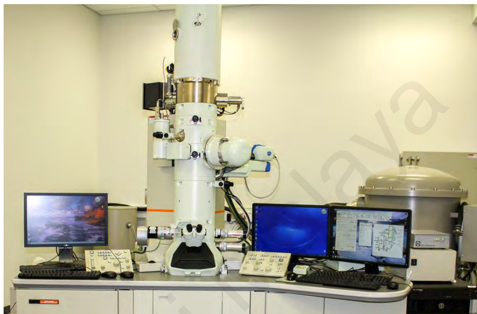
Figure 3.7: High resolution transmission electron microscope Jeol JEM-2100F.
