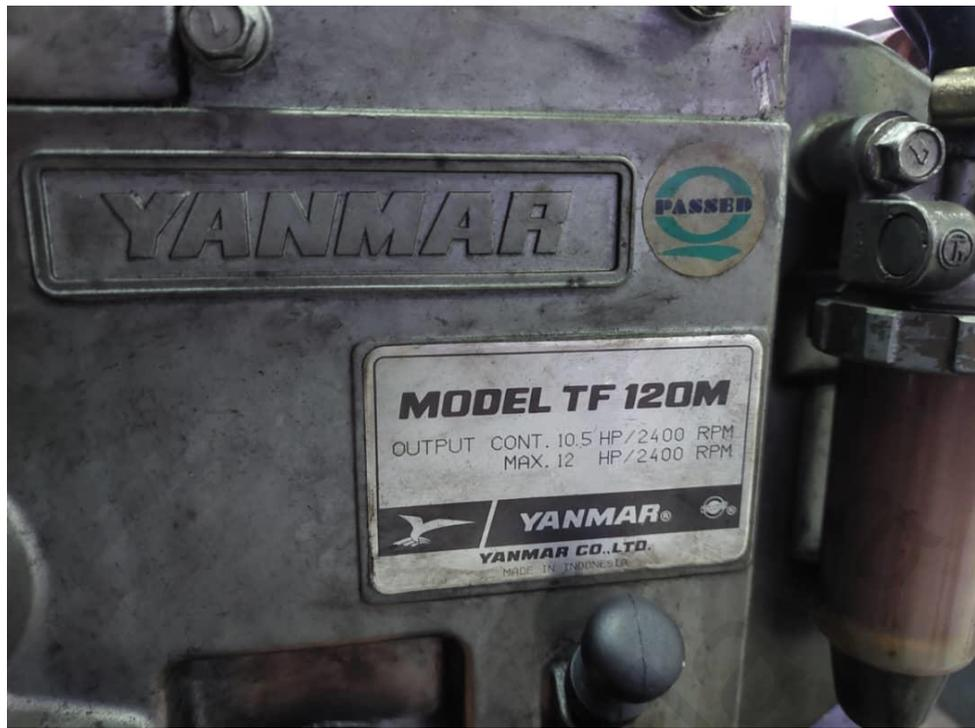
**Figure 15: Test Engine Manufacturer Specifications**
