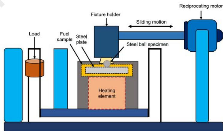
**Figure 11: HFRR Test Setup**
