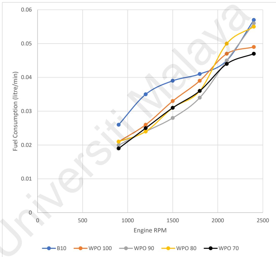
**Figure 25: Graph of Fuel Consumption (Litre/min) for Various Fuel Samples**
