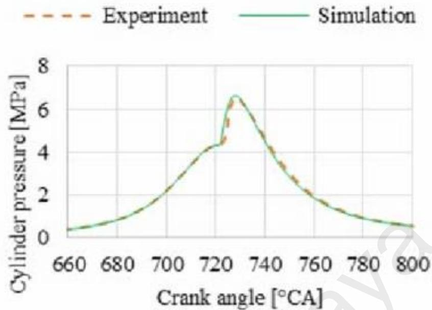
**Figure 4: Cylinder Pressure in a Common Diesel Engine**
