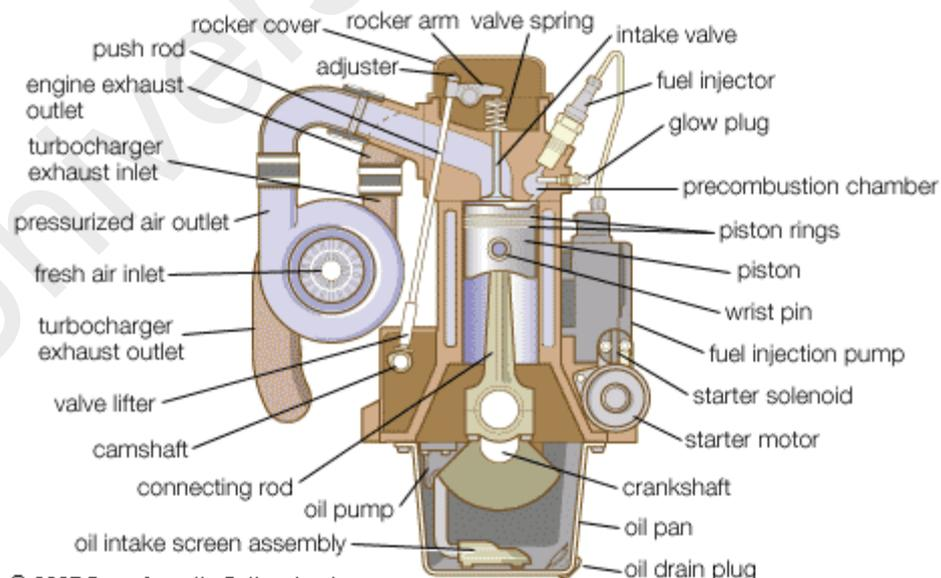
**Figure 2: Typical Layout of a Modern Diesel Engine**
