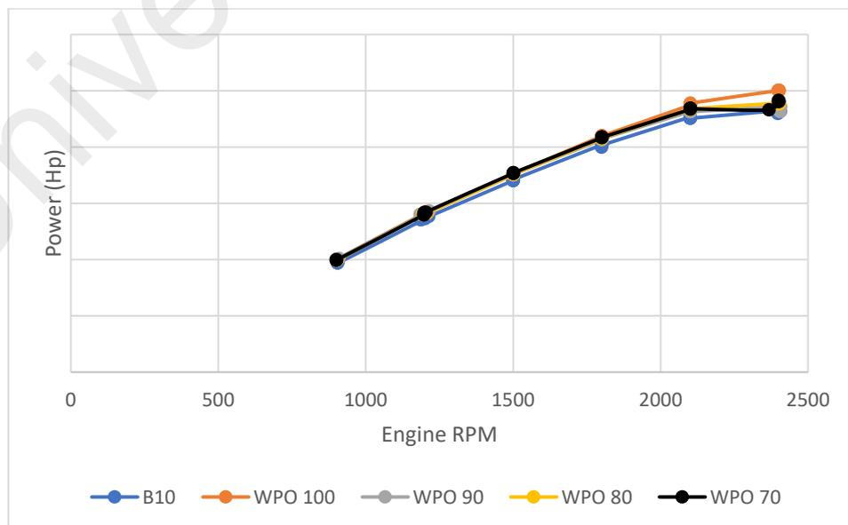
**Figure 23: Graph of Power (Hp) against RPM for Various Samples**
