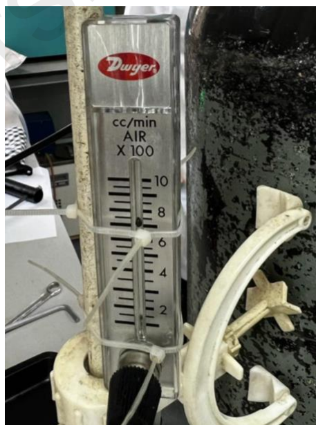
Figure 3.3: The nitrogen gas flow adjusted at 7 cc/min
