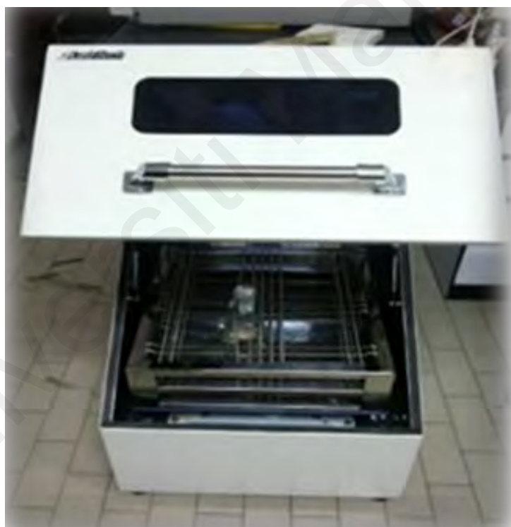
Figure 3.5: The batch fermentation of biohydrogen using an incubator shaker.
