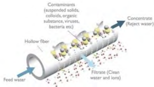
Figure 2-2: Hollow fiber Ultrafiltration system mechanism.
