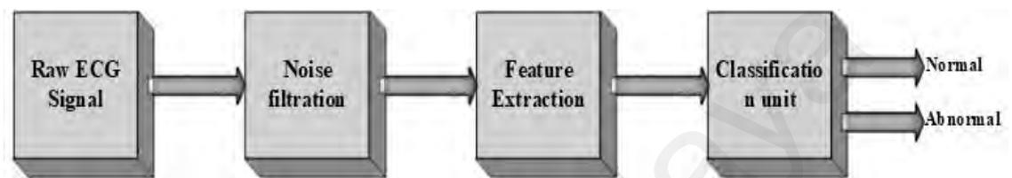
**Figure 2.4. Block model of the primary ECG classification process**
