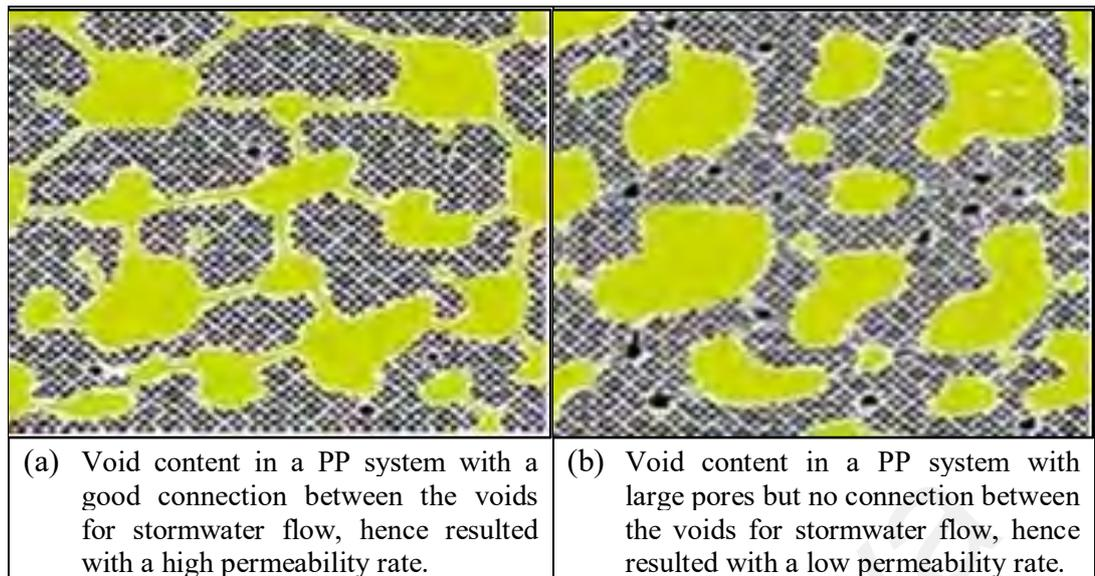
**Figure 2.12: Permeable pavement with (a) interconnected pores, and (b) loss of connection due to surface clogging**
