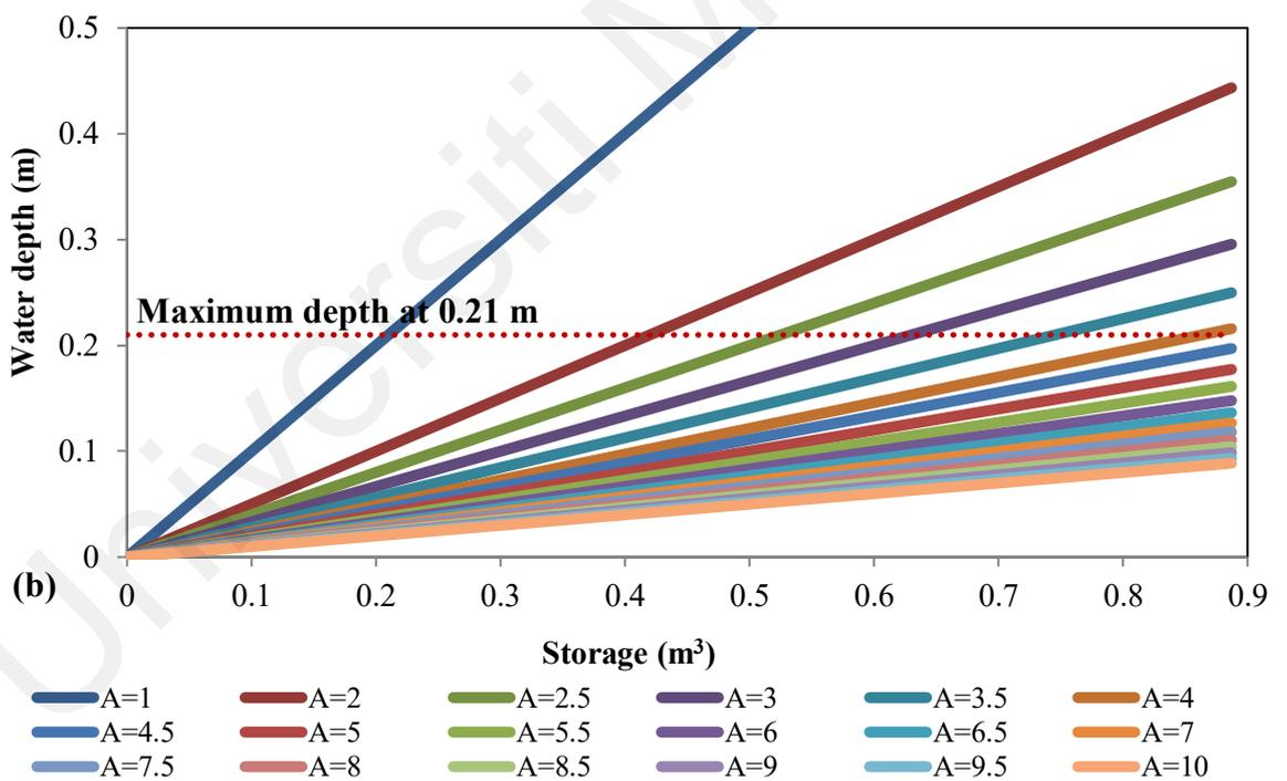
**Figure 4.8: Relationship between (a) water depth and duration, and (b) water depth and storage capacity for different coverage areas**
