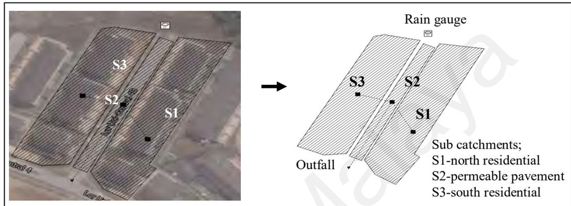
**Figure 3.20: Subcatchments, consisting of S1 (north residential), S2-permeable pavement, and S3 (south residential)**
