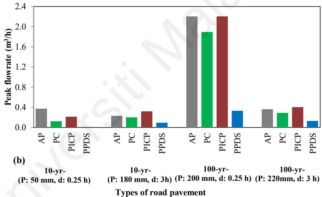
**Figure 4.16: Performances in terms of (a) runoff coefficients and (b) peak flow for each simulated pavement under rainfall events of 10-yr and 100-yr ARI**
