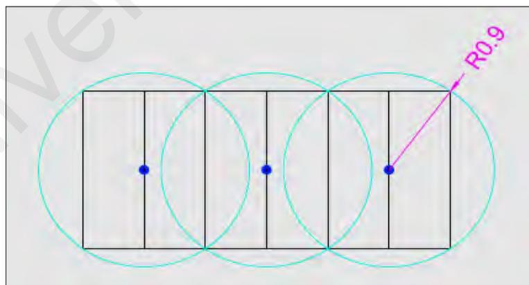
**Figure 3.6: Nozzle coverage area of the green pavement box**
