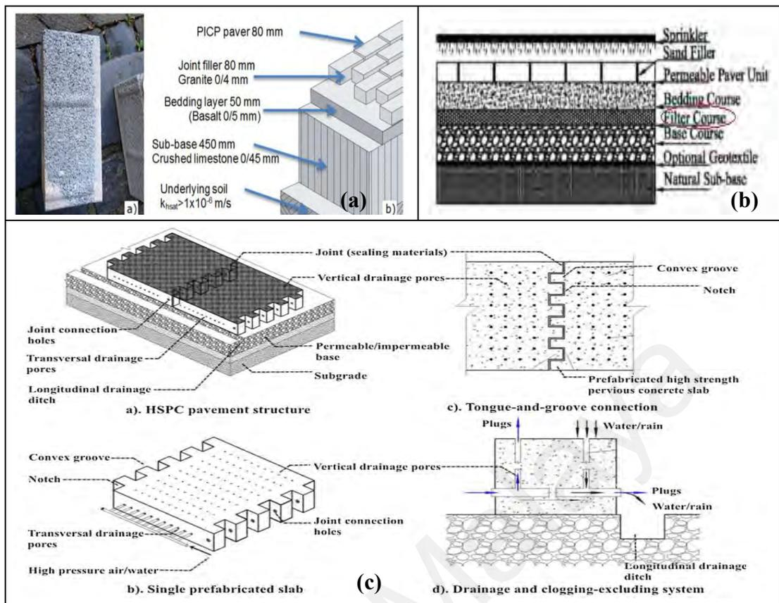
**Figure 2.15: New design of permeable pavement proposed by (a) Dierkes & Lucke (2015), Lucke & Dierkes (2015) and Lucke (2014), (b) Imran et al. (2013), and (c) Li et al. (2017)**
