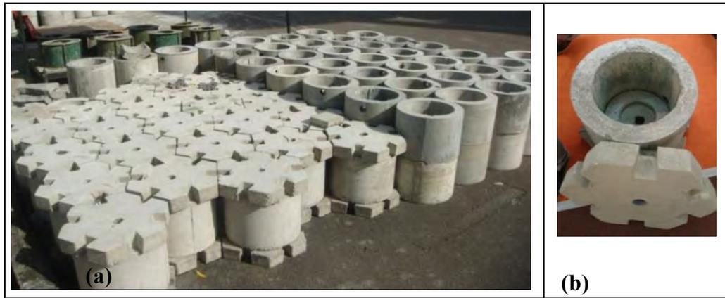
**Figure 3.3: PPDS system: (a) arrangement of PPDS assembled outside the laboratory, and (b) PPDS precast product single unit of a hollow cylinder and cover design**
