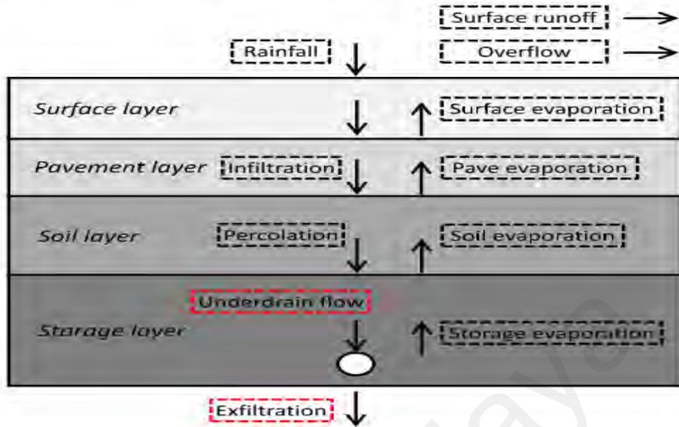
**Figure 2.13: Schematic diagram showing the conceptual model of LID practice in SWMM (Source: Zhang et al., 2018)**
