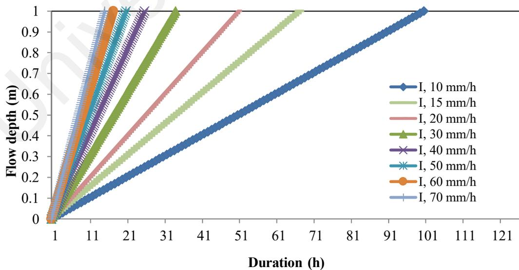
**Figure 4.12: Permeability performance of PPDS with respect to the different infiltration rates**
