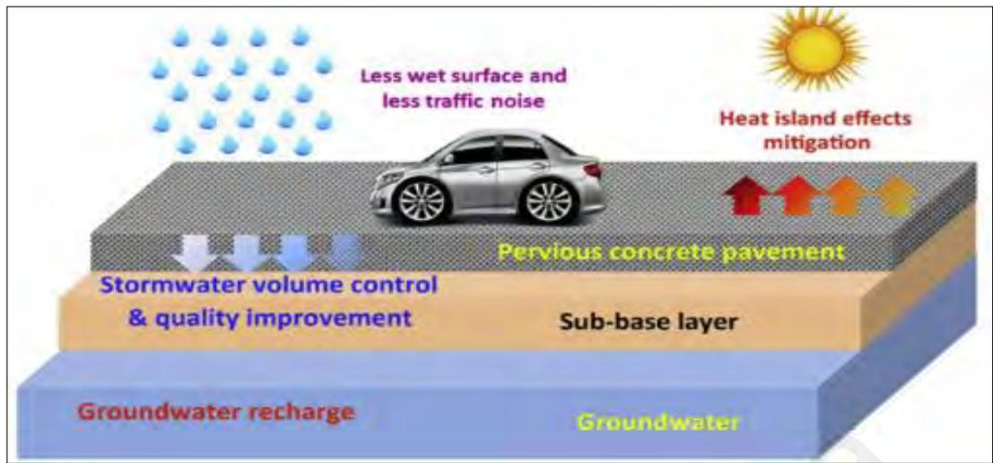
**Figure 2.6: Stormwater management benefits while applying permeable pavement (Source: Xie et al., 2019)**
