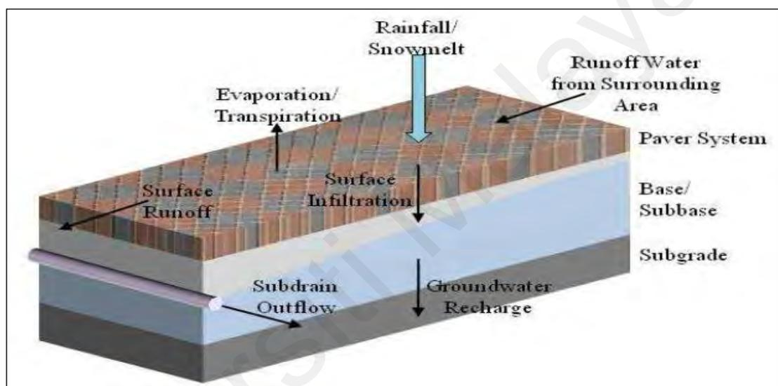
**Figure 2.9: Inflow and outflow of water on the permeable pavement (Source: Swan & Smith, 2009)**
