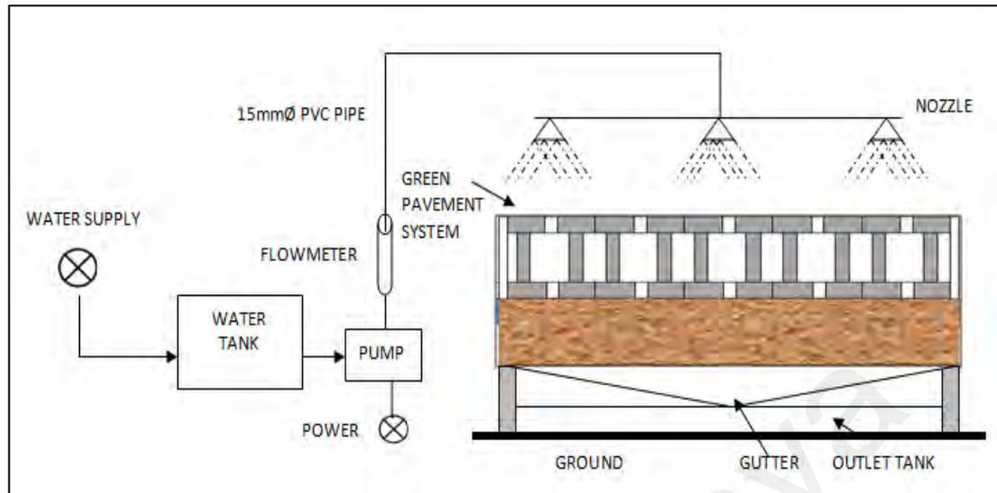
**Figure 3.5: Graphical design of the rainfall simulator**
