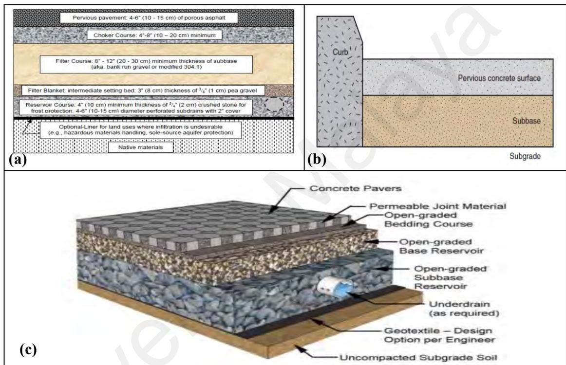
**Figure 2.11: Typical cross-section of permeable pavement system (a) porous asphalt pavement (NAPA, 2008), (b) pervious concrete pavement (Source: ACPA, 2009) and (c) permeable interlocking concrete paver system (Source: ICPI, 2013)**
