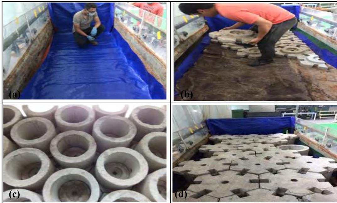
**Figure 3.14: Experimental set up to investigate storage capacity of PPDS system**
