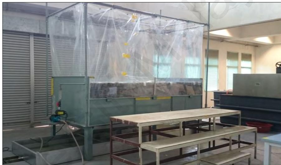
**Figure 3.9: Rainfall simulator in the hydraulic laboratory for PPDS experimentation**
