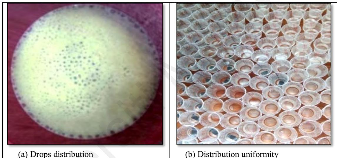
**Figure 4.1: Calibration on (a) drop sizes, and (b) distribution uniformity.**
