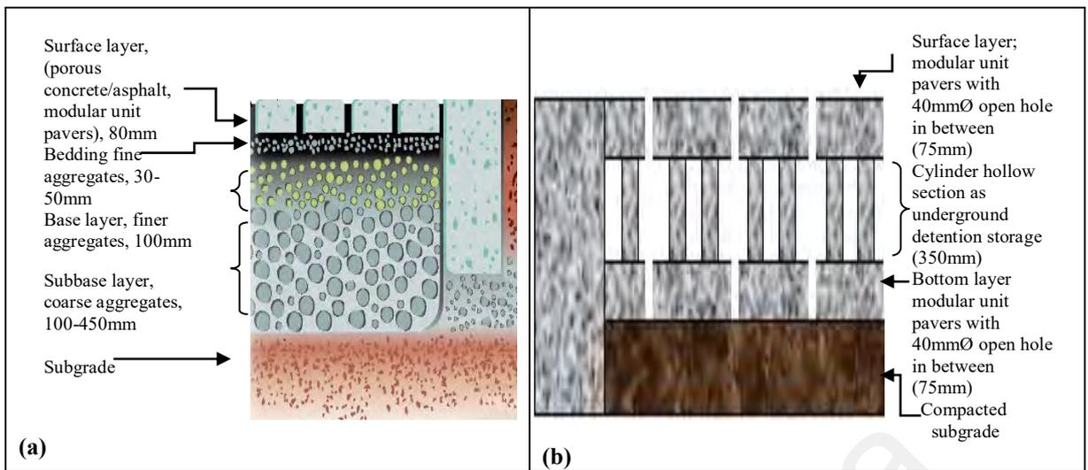
**Figure 3.4: Cross-section design of (a) typical permeable pavement, and (b) suggested PPDS**
