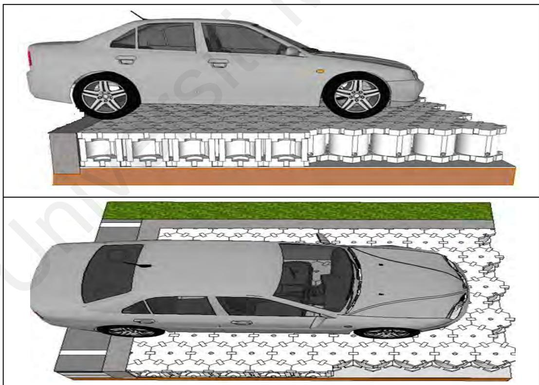
**Figure 1.1: Conceptual design of modified stormwater management infrastructure, PPDS with interlocking pavers (Source: Bateni et al., 2019).**
