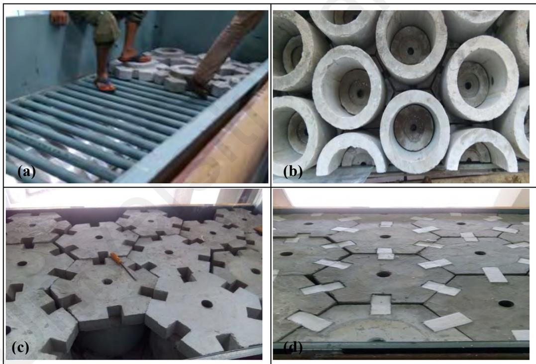
**Figure 3.13: Experimental set up to investigate permeability rate of PPDS system**
