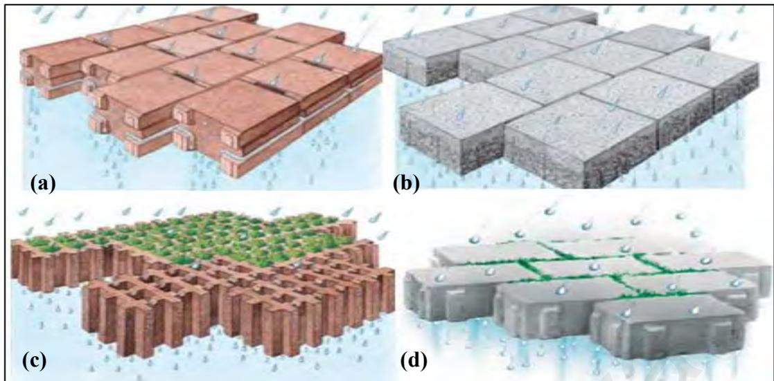
**Figure 2.2: Permeable pavement systems: (a) pavers with canals, (b) porous pavers, (c) small apertures, and (d) wide joints (Source: Dierkes et al., 2000, 2002)**
