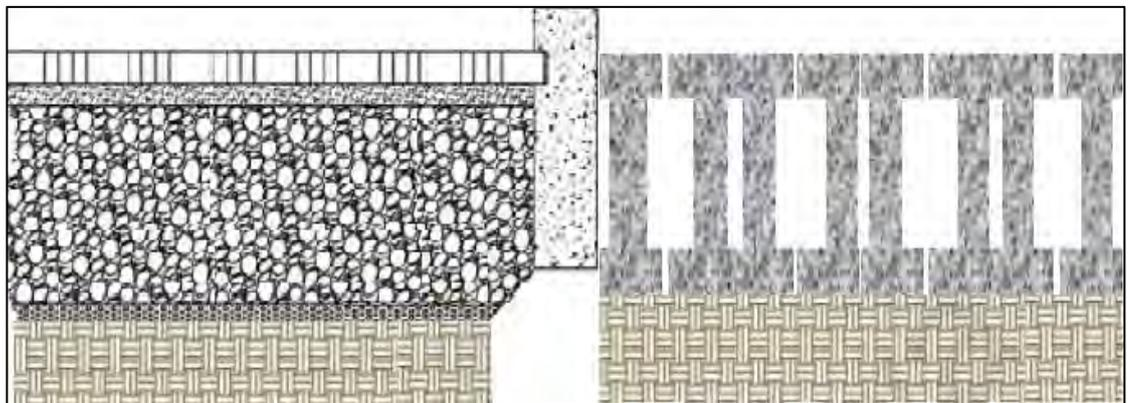
**Figure 2.17: Cross-section of, (a) typical PICP pavement structure, and (b) new green pavement design, permeable pavement with micro detention storage (PPDS)**
