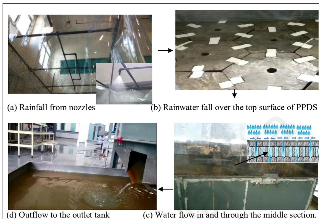
**Figure 3.12: Flowpath of the rainfall in the rainfall simulator and through the PPDS system**
