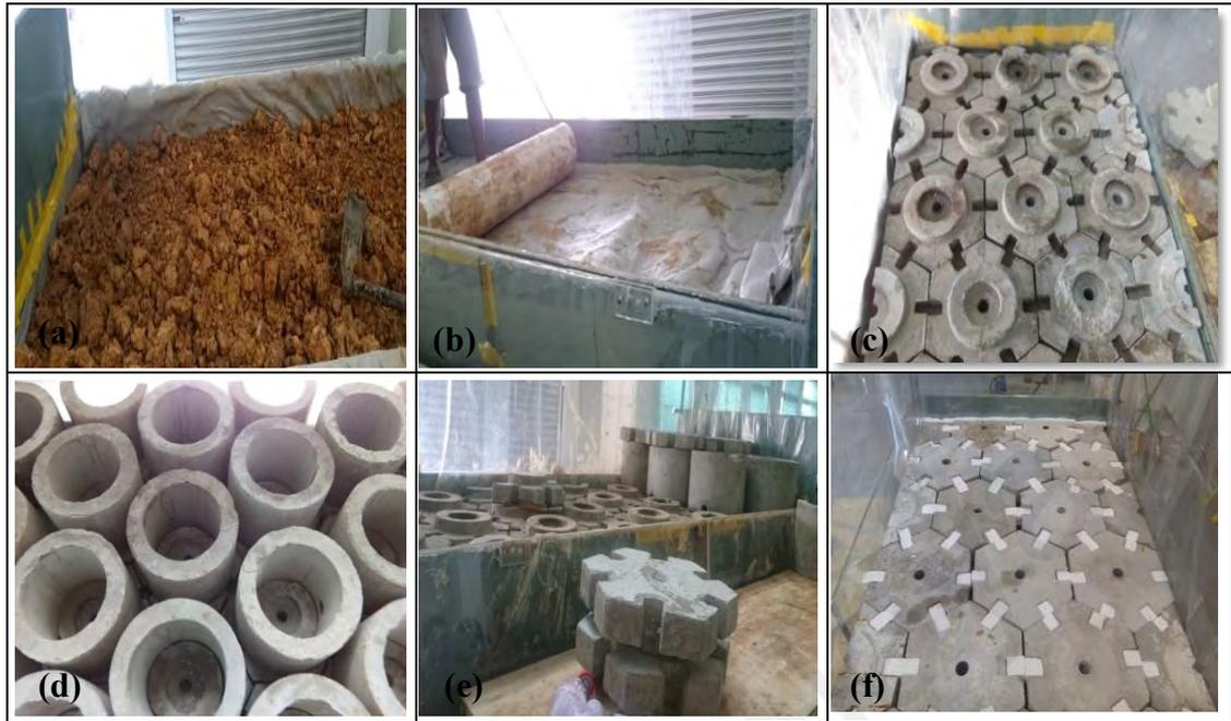
**Figure 3.15: Experimental set up to investigate storage capacity and infiltration rate of PPDS system**
