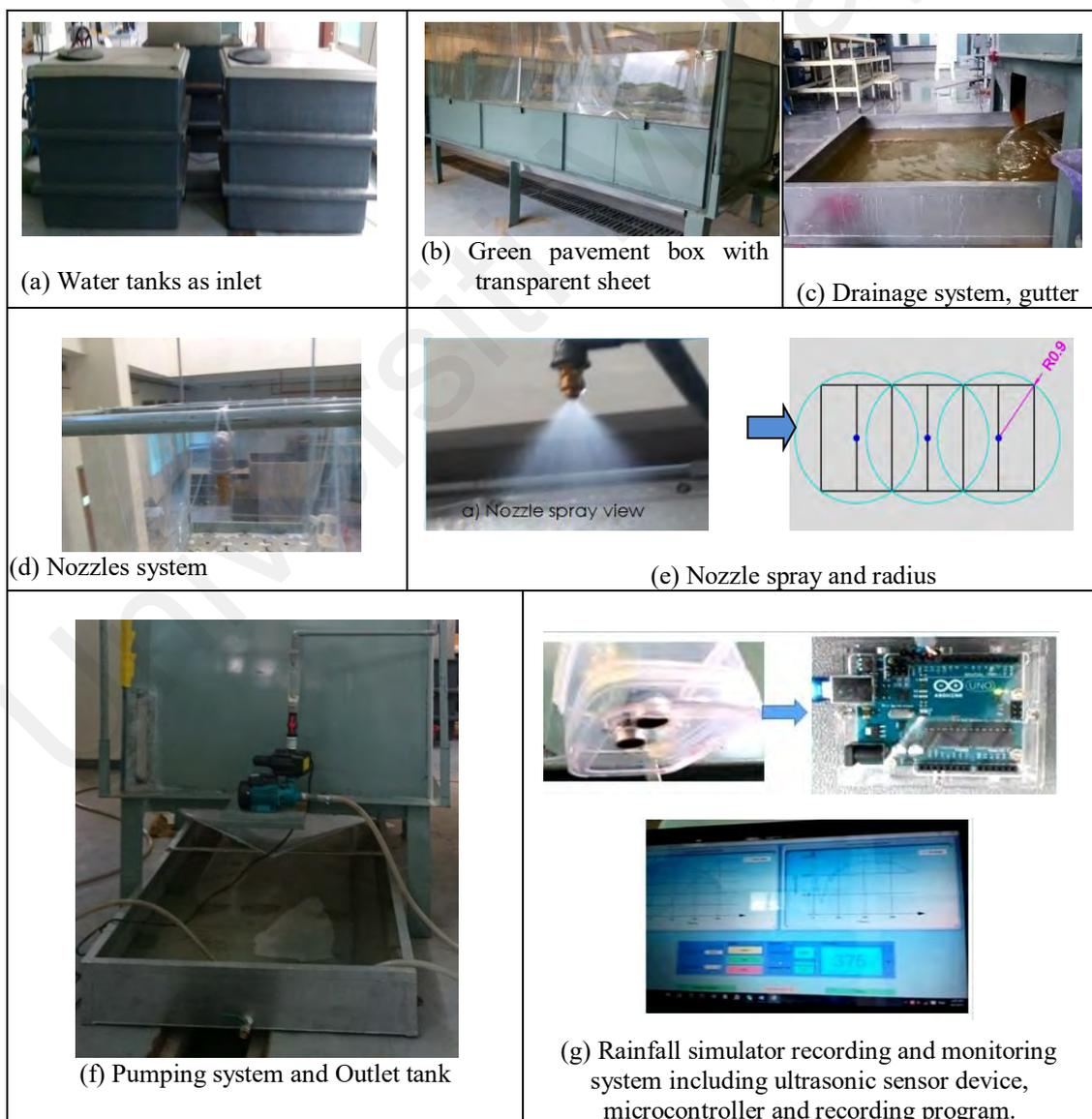
**Figure 3.10: Components of rainfall simulator at the laboratory**
