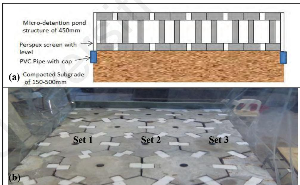
**Figure 3.7: Green pavement box: (a) cross-section of PPDS system with subgrade, and (b) PPDS arrangement, with 3 sets per column**
