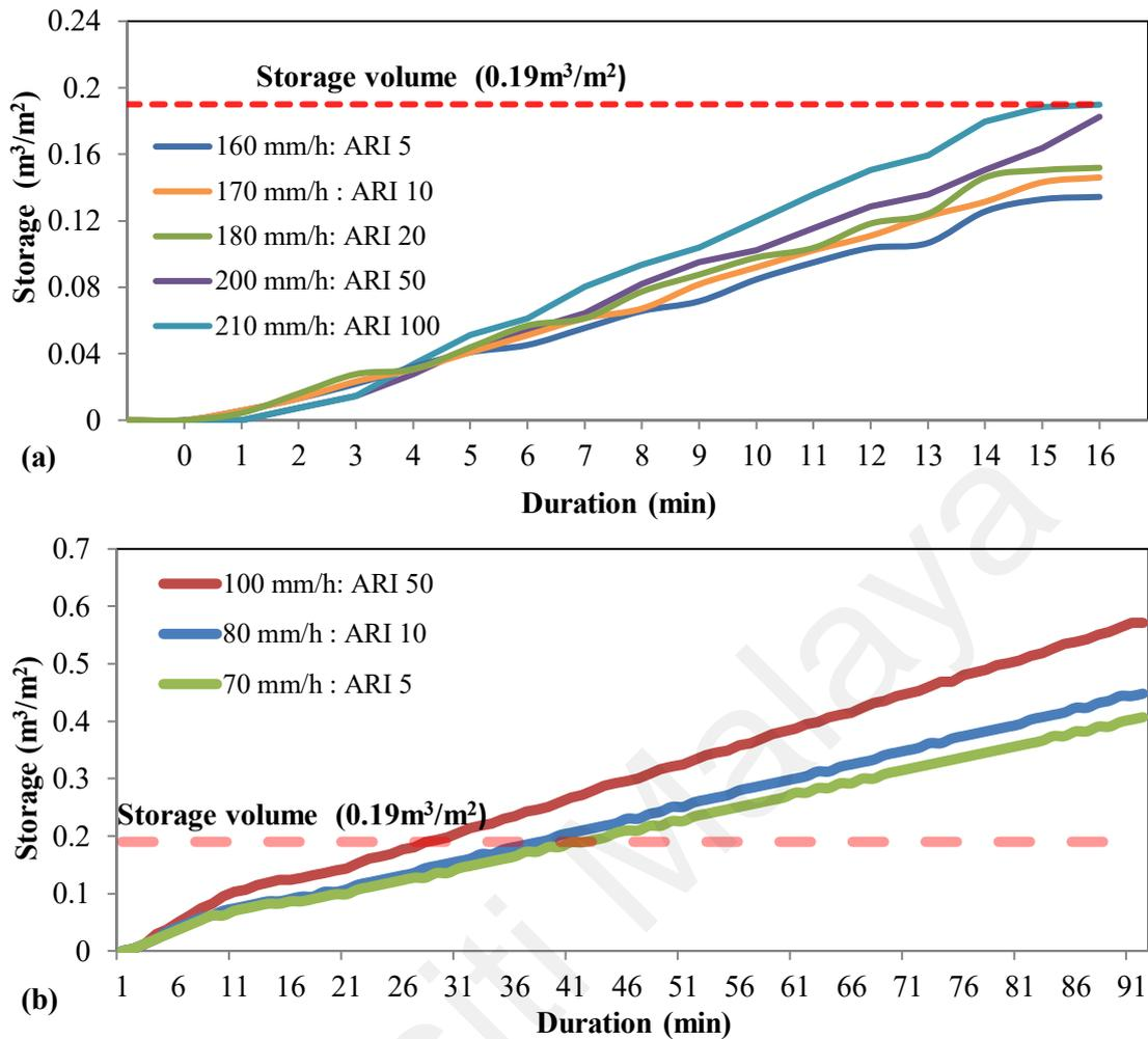
**Figure 4.6: Storage volume of PPDS with duration at various rainfall intensity for (a) 15-minutes rainfall duration, and (b) 90-minutes rainfall duration**
