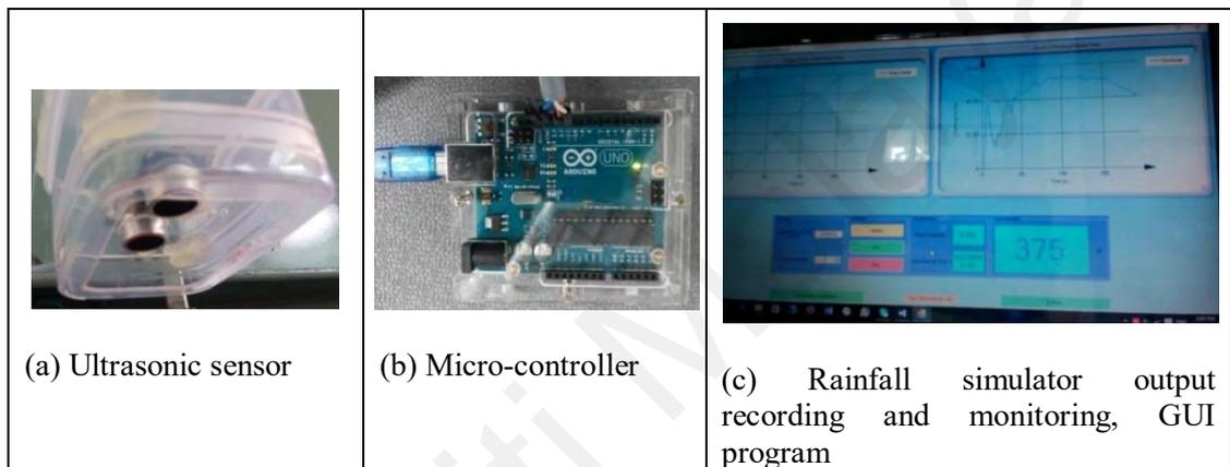
**Figure 3.8: Output device for recording and monitoring of outlet discharge**
