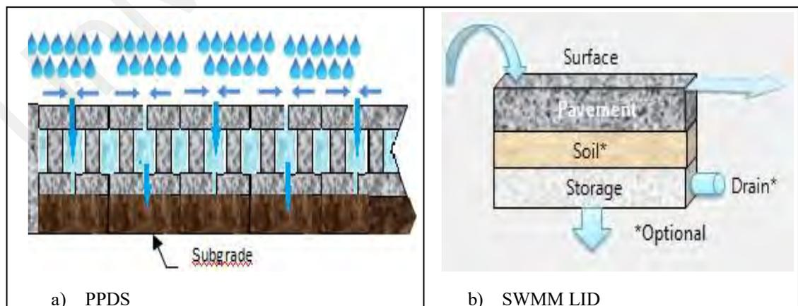
**Figure 3.17: Schematic diagram of the rainfall route in the system**
