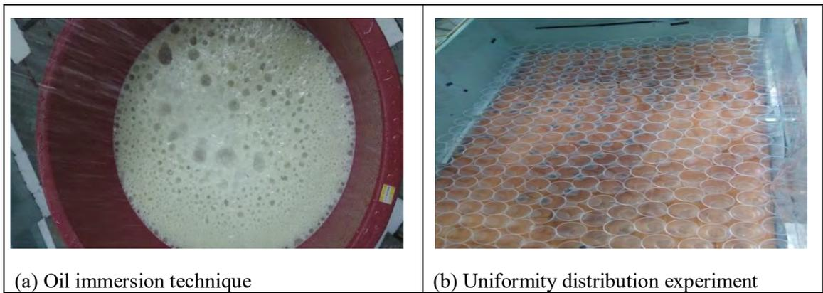
**Figure 3.11: Calibration of the rainfall simulator: (a) oil immersion technique, and (b) distribution uniformity over the catchment area**
