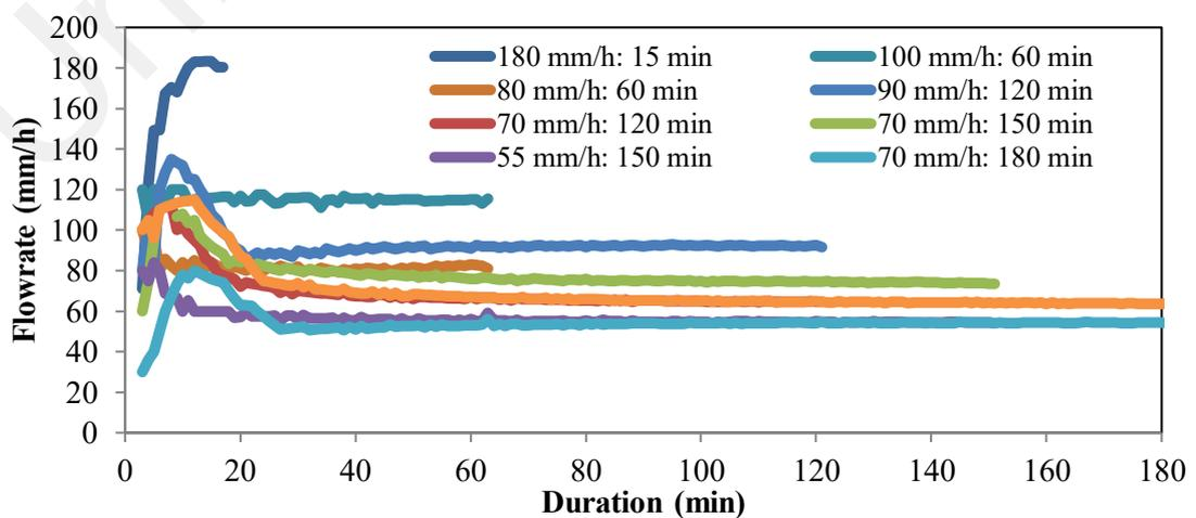
**Figure 4.4: Flow pattern in PPDS with duration, at various rainfall intensities**
