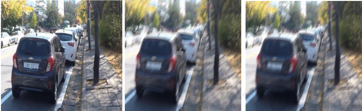
Figure 3.2 Sample of images. (a) Ground truth image. (b) Blurry image generated by convolving a uniform blur kernel. (c) Blurry image by averaging sharp frames.
