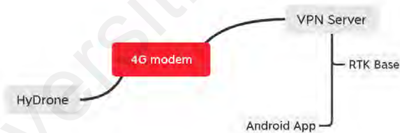
Figure 3.35: Internet-Connected over a 4G modem
