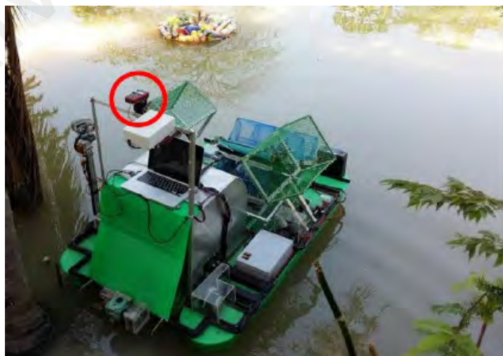
Figure 2.9: The floating waste scooper robot (Ruangpayoongsak et al., 2017)
