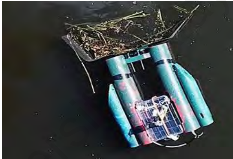
Figure 2.4: Garbage-cleaning robot (Abrams, 2018)
