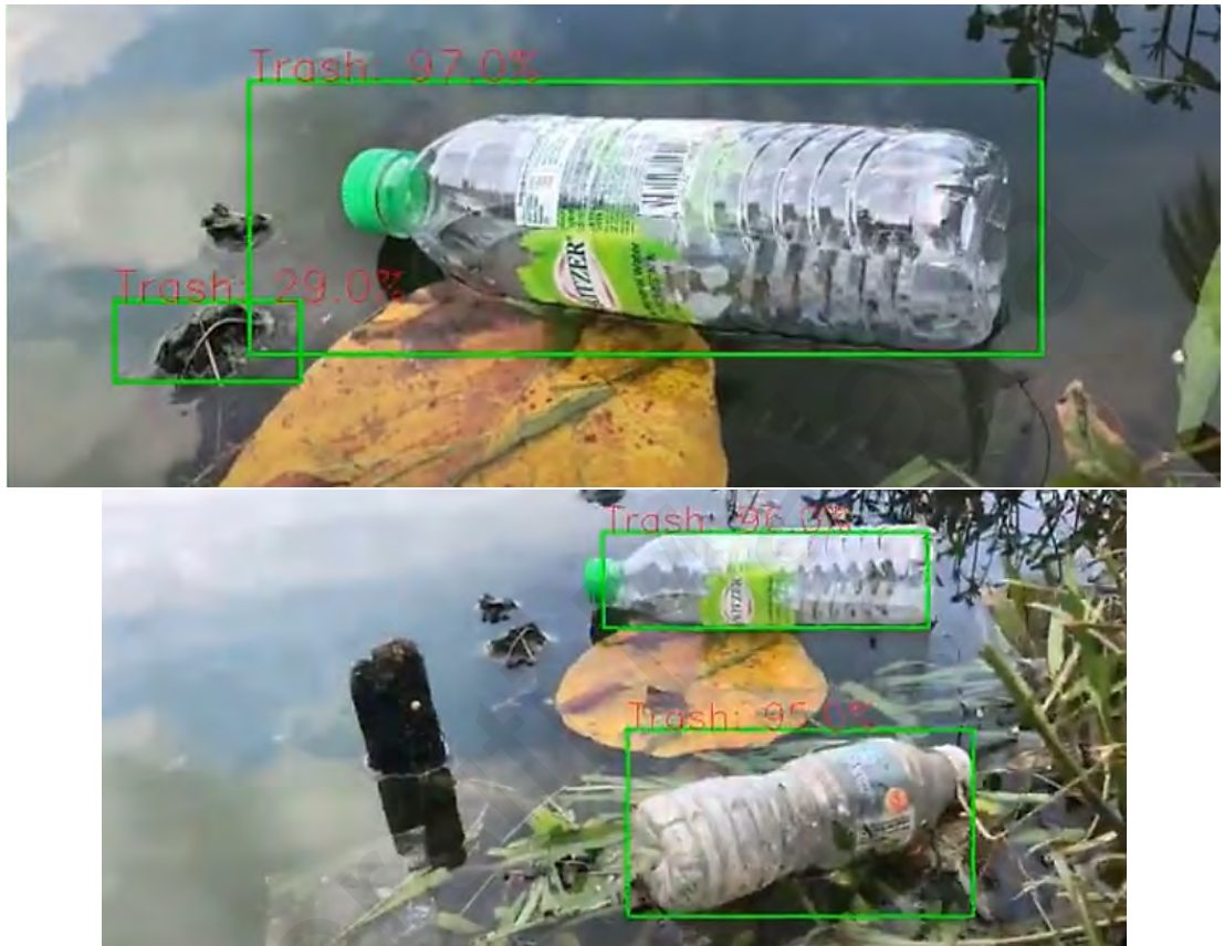
Figure 4.32: Accurate detection when floating garbage is near and static
