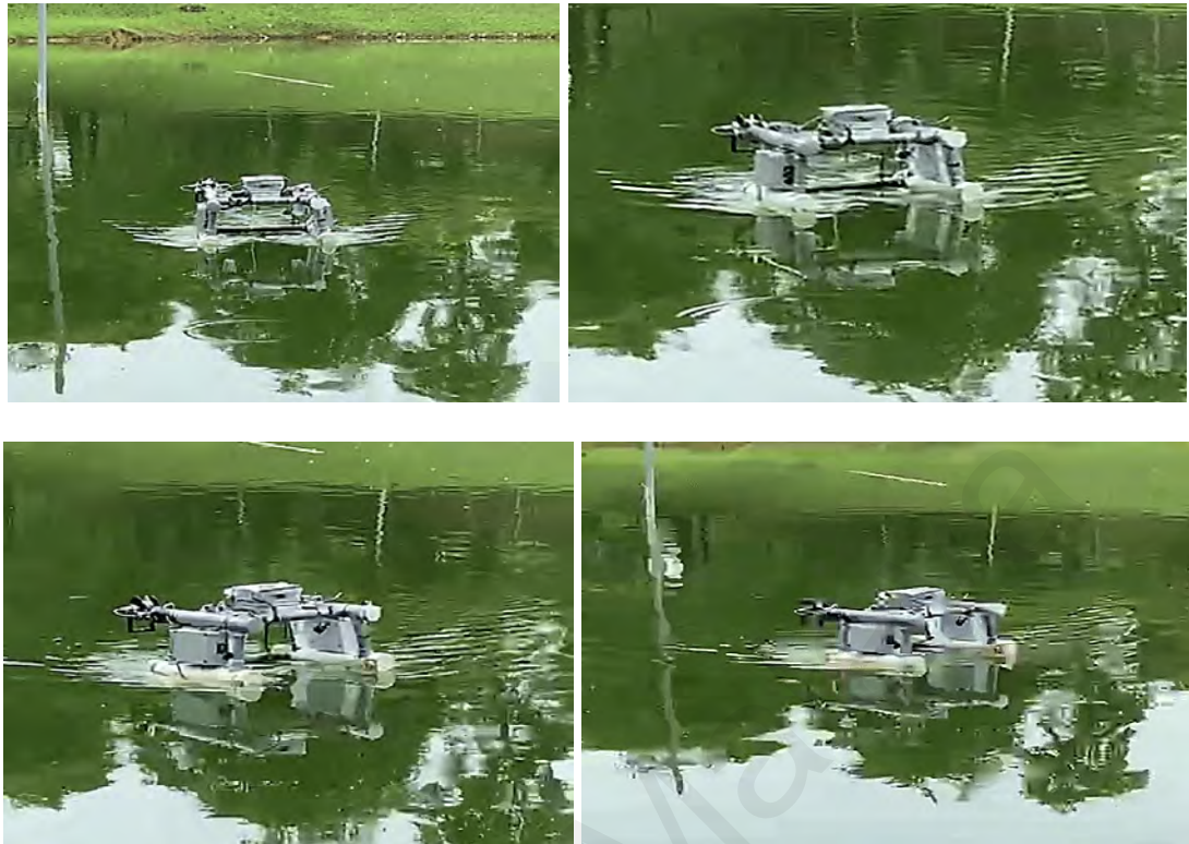
Figure 4.28: Robot turning at each station to direct heading towards the next target
