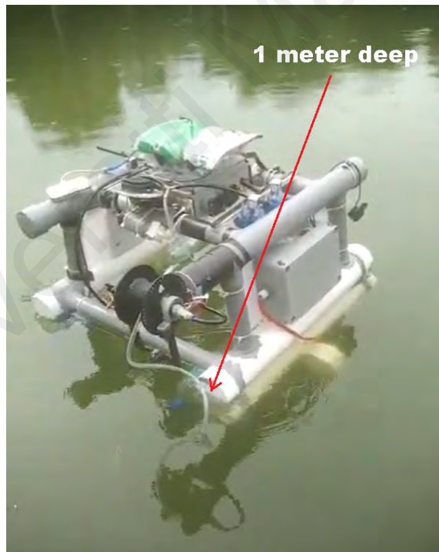
Figure 4.8: Underwater sampling (1-meter depth) conducted at the UM lake
