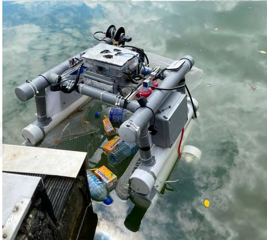
Figure 4.35: Nylon net trapping floating garbage from sanitation task
