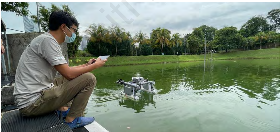
Figure 4.12: Driving robot remotely using the Android mobile app
