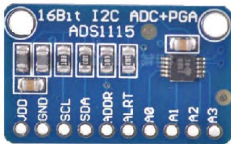
Figure 3.21: 16bit ASD1115 and Logical level converter
