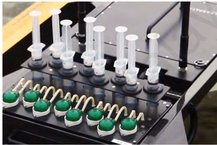
Figure 2.19: Sampler syringes Heron USV (Clearpathrobotics, 2016)
