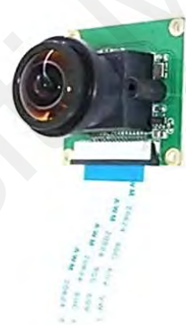
Figure 3.18: 5 megapixel Raspberry Pi camera with its 3D casing design
