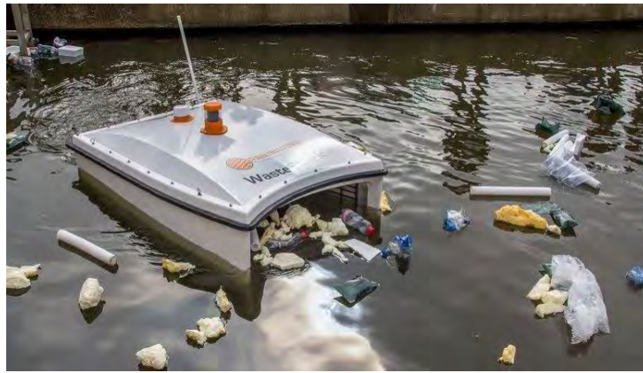
Figure 2.10: The WasteShark (Blue Growth, 2018)
