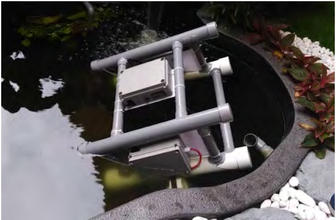
Figure 4.2: Early day testings when buoyancy not achieved
