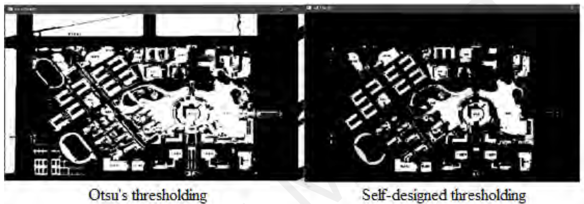
Figure 3.8: Non-bimodal image thresholding
