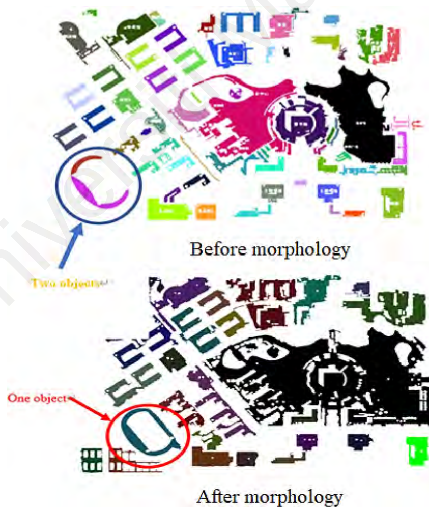
Figure 3.12: Example of using morphology in resolving disconnected object
