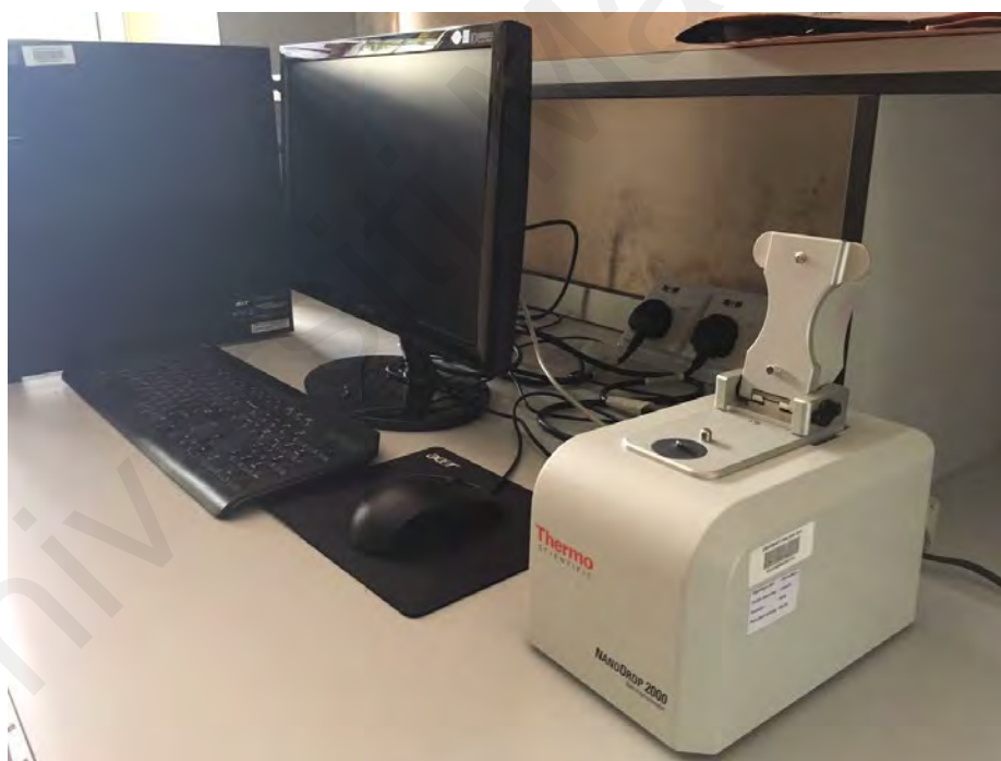
Figure 3.2: The NanoDrop spectrophotometer used in this research (Institute of Biological Sciences, Faculty of Science, University of Malaya).
