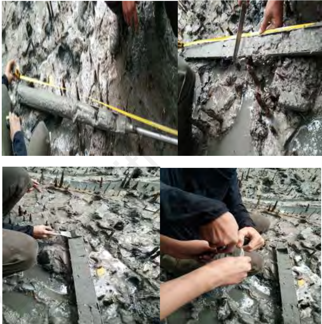
Figure 3.4: collection of soil sample from an open face auger
