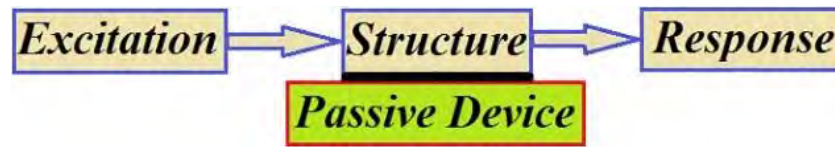
Figure 2.8: Components of PVC system
