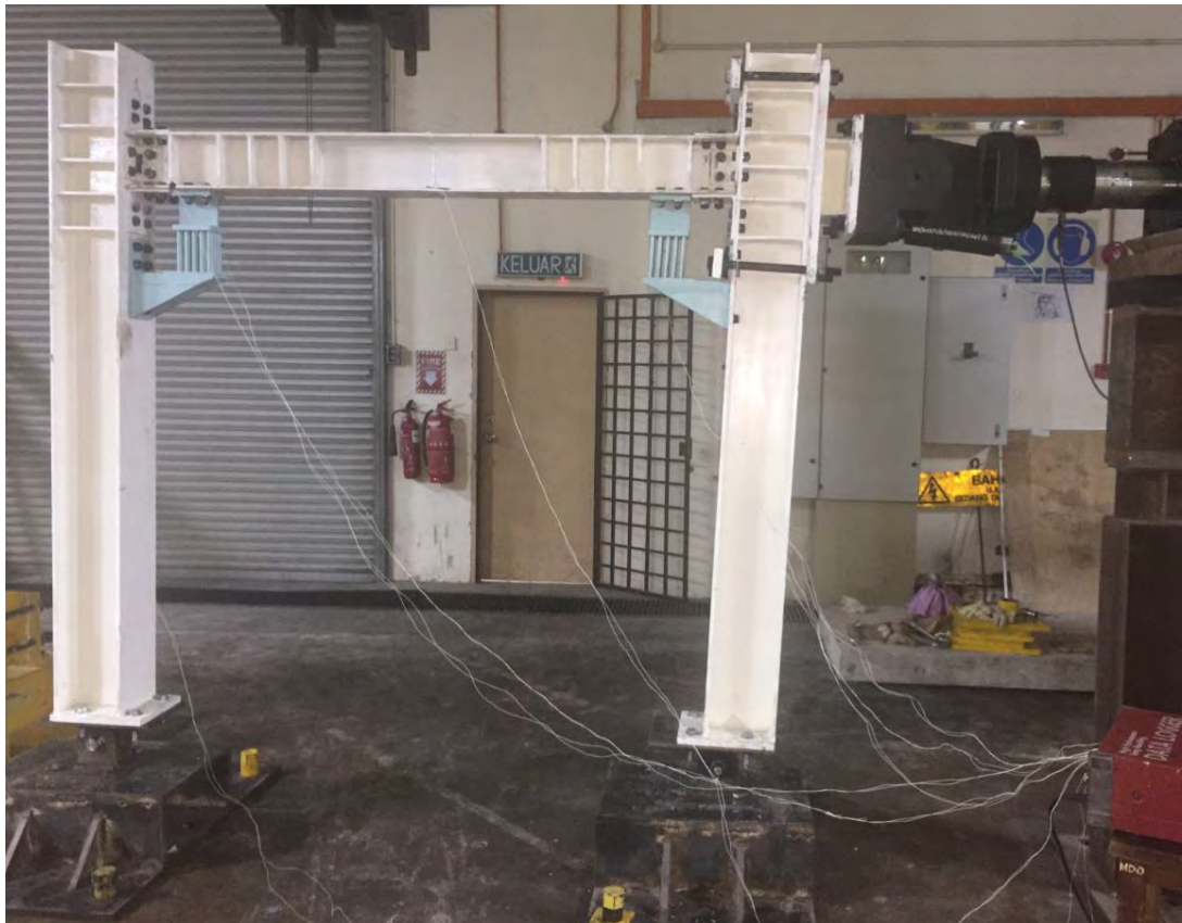
Figure 5.9: Test setup of the frame with BD
