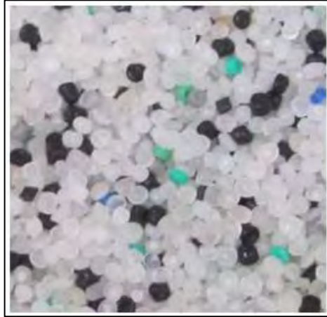
Figure 2.25: Regenerate particles mixed with different color particles (Jiao & Sun, 2016)
