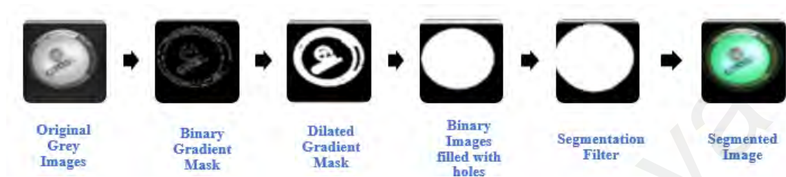
Figure 3.13: Segmentation stages for bottle class sample
