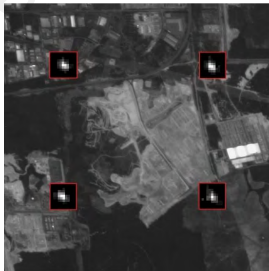
Figure 1.4: Example of a satellite image with a spatially varying blur; The red boxes emphasize the close-up view of the spatial varying blur kernel of the satellite image.
