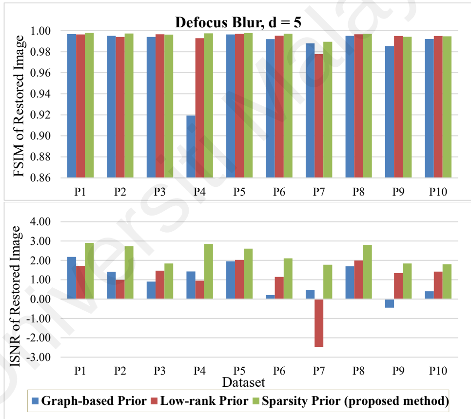
Figure 5.9: Quantitative evaluation for defocus blur, d = 5 in terms of ISNR, and FSIM on all datasets.
