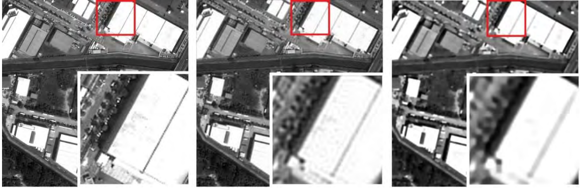
Figure 6.1: Comparison of visual quality for image restoration in different domains. The red box denotes the cropped region. (a) Original Image, (b) Restored image by Wiener filter (Lee et al., 2016), illustrating the rise of ringing effect and noise amplification, and (c) Restored image by Anisotropic TV model (Pan et al., 2017), illustrating over smooth effect that created an unnatural appearance.
