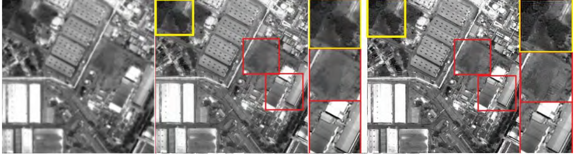
Figure 6.8: Effectiveness of the proposed prior, the block regions show the cropped region and their closed-up view. (a) Blurred-noisy input (gaussian blur, \sigma = 2 ), (b) intermediate latent image f_L restored by Equation (6.7). (c) Restored results using the method by Krishnan & Fergus (2009). The closed-up view from the yellow box obviously shown boundary artifacts.
