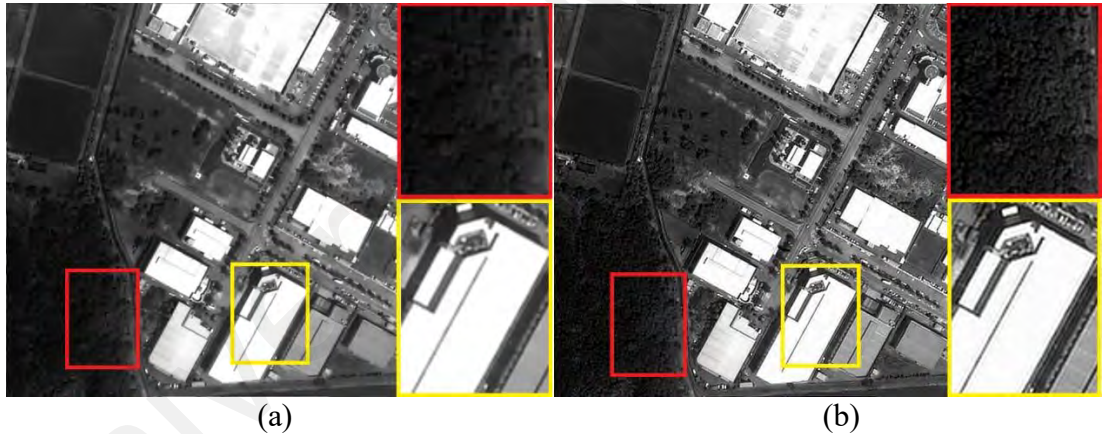
Figure 6.2: Comparison of visual quality for image restoration in different domains. The yellow and red boxes denote the cropped regions. (a) Restored image using anisotropic TV-prior (Pan et al., 2017); As can be seen there are no visible noise and ringing artifacts in the cropped regions, but the forest tree and the roof are too smooth. (b) Restored image by Laplacian prior (Oh and Choi, 2014); as can be seen that the cropped regions are rich in detail, however, they also exhibit a few ringing artifacts.
