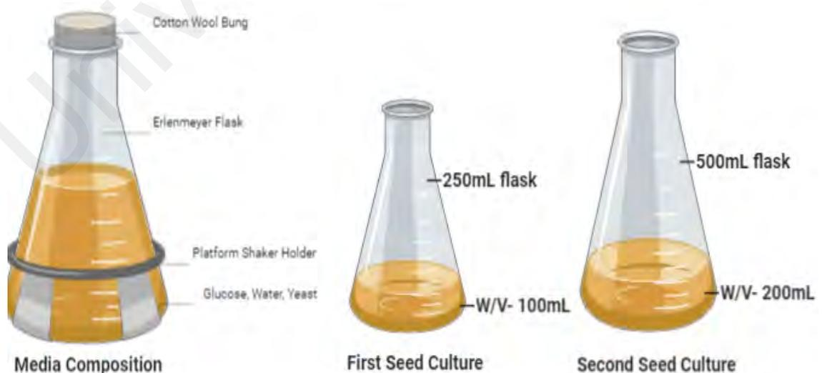
**Figure 2.4: Basic apparatus of a laboratory-scale submerged fermentation (figure by author)**
