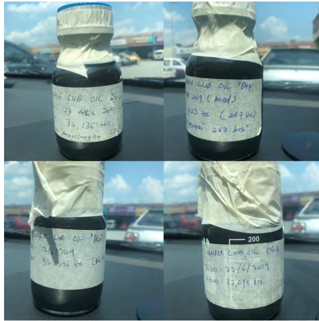
Figure 3.9: Oil Samples Collected for Oil Analysis.
