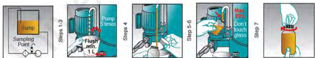
Figure 3.8: Steps for oil sampling
