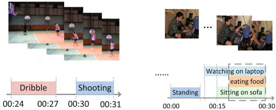
Figure 4.7: Different temporal definition of events in videos for a single event (left) and multiple events with overlap (right) (Mleya et al., 2019).
