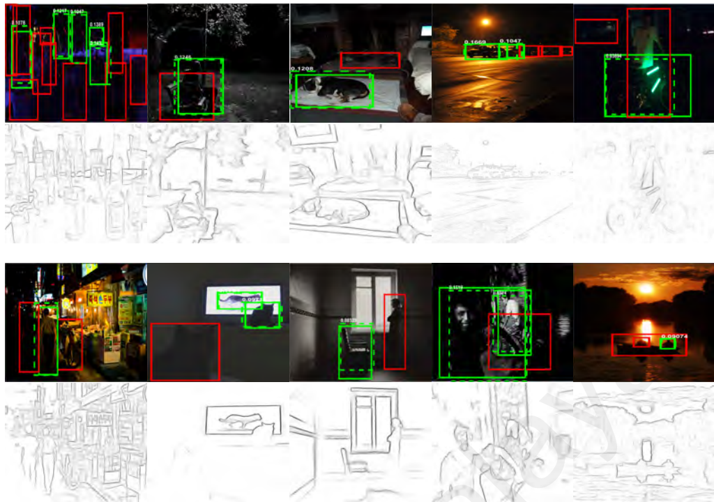
Figure 4.12: Examples of Edge Boxes proposals (Max. proposals = 1000; IoU = 0.7) on different types of low-light images and visualizations of the edge features. (Red: undetected groundtruth; Green: detected groundtruth, Green dotted: proposed box) From left, first row: Low, Ambient, Object, Single, Weak; second row: Strong, Screen, Window, Shadow, Twilight.
