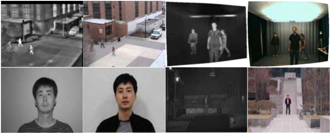
Figure 2.1: Top row: Examples of thermal images and their corresponding images captured in visible light. Bottom row: Example images of a person at short (1m) and long (150m) distances captured using NIR in low-light and using digital camera in bright environment.
