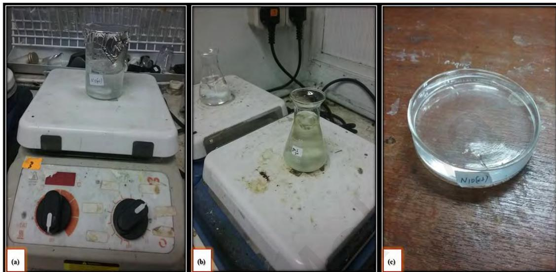
**Figure 3.1: (a), (b) and (c) System A [PAAC-NaI] solutions stir uniformly with magnetic stirrer and the casted solution after stir 24 hours respectively.**
