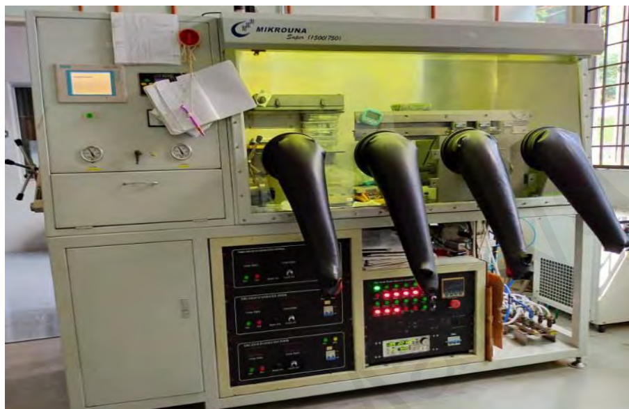
Figure 3.3: The nitrogen-filled glove box by MIKROUNA Super (1500/750).
