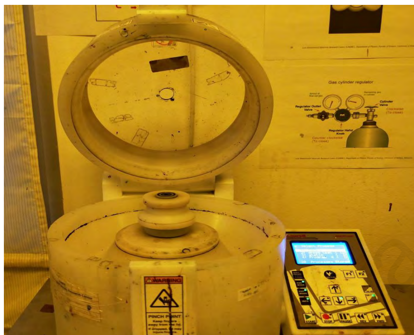
Figure 3.4: Spin coater by Laurell model WS-650MZ-23NPP.
