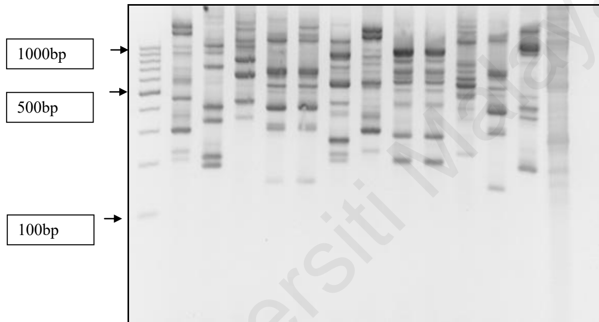
Figure 4.6 Agarose electrophoresis of BOX-PCR gels. Lanes labeled M was run with the DNA size standard (100bp ladder; Fermentas Corp.), sizes of fragments (bp) are indicated on the left. Lane 1, isolate TY046-021; lane 2, TY028-047; lane 3, TY046-016; lane 4, TY046-071; lane 5, TY046-078; lane 6, TY046-017; lane 7, TY046-027; lane 8, TY046-073; lane 9, TY049-057; lane 10, TY029-014; lane 11, TY047-019; lane 12, TY028-043; lane 13, TY029-008; lane 14, negative control.
