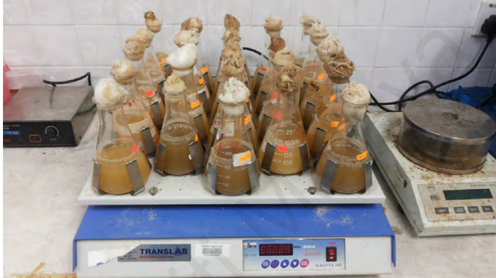
Plate 3.3: All samples were put onto the orbital shaker at 150 rpm in room temperature for 8 days.
