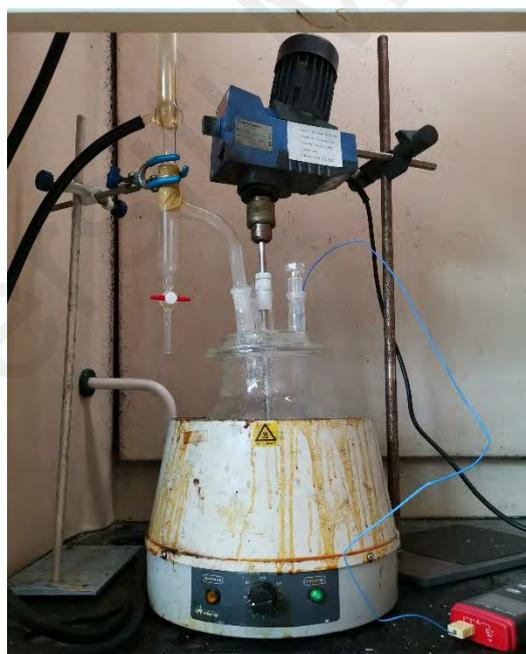
**Figure 3.11: Experimental setup during polyesterification stage**
