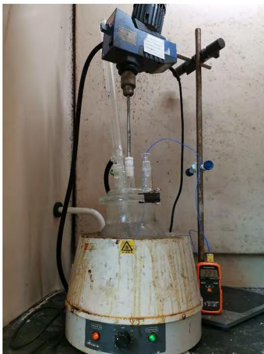
**Figure 3.10: Experimental setup during alcoholysis stage**
