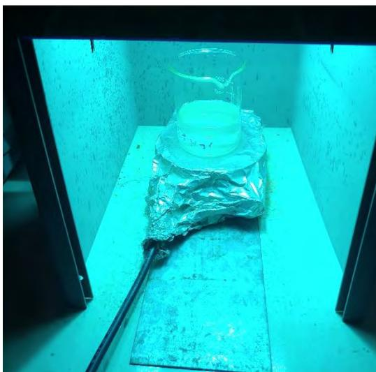
**Figure 3.1: UV irradiation of ENR25 in THF solution**
