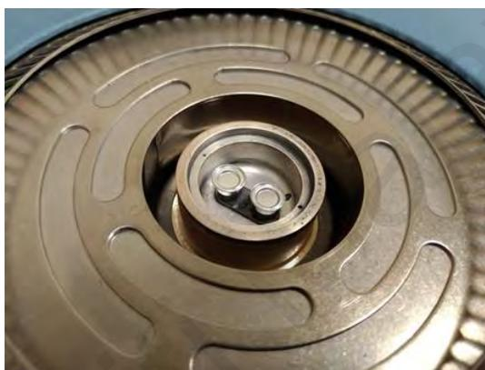
**Figure 3.5: Heat flux DSC with single furnace which accommodate both sample pans**
