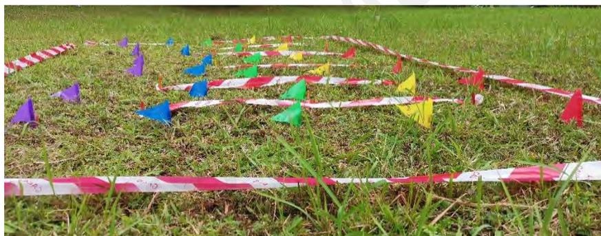
**Figure 3.9: Outdoor soil burial method of biodegradability test**
