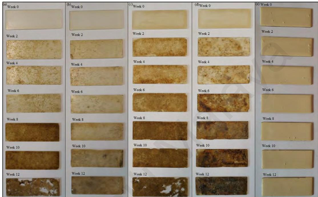
**Figure 4.24: Photographs of (a) Coating T10 (in lab), (b) Coating T10 (open environment), (c) Coating T35 (in lab), (d) Coating T35 (open environment) and (e) Coating Epo (in lab) from week 0 to week 12 throughout biodegradation process**
