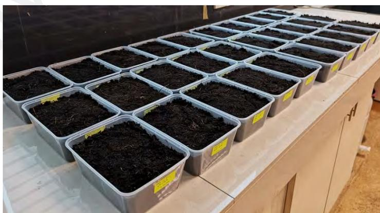
**Figure 3.8: Indoor set of soil burial method of biodegradability test**
