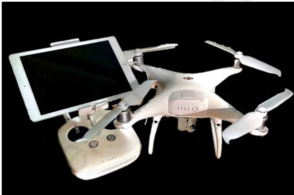
Figure 3.2: DJI Phantom Pro 4 (FOV 84° 8.8 mm/24 mm, f/2.8 - f/11 auto focus at 1 m - ∞, 100 - 3200 (Auto)) with iPad Apple for disease aerial monitoring.
