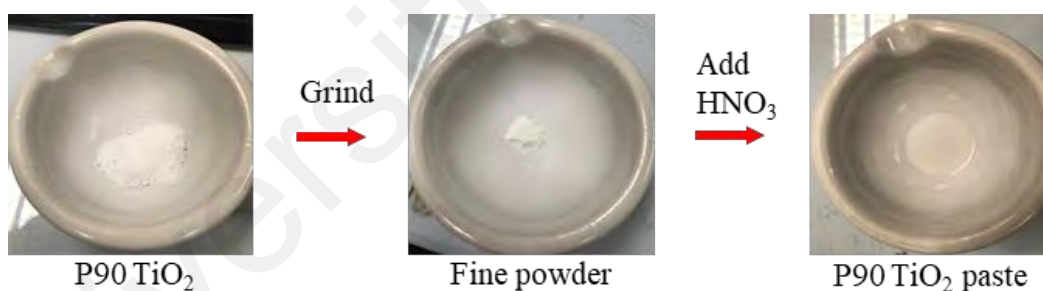
Figure 3.9: Preparation of P90 TiO 2 paste.
