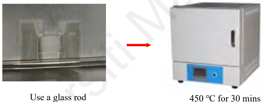
Figure 3.12: Deposition method of P25 TiO 2 paste on the surface of FTO glass.
