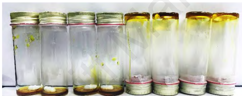
Figure 4.8: Texture of W0 (from left) to W7 GPE.
