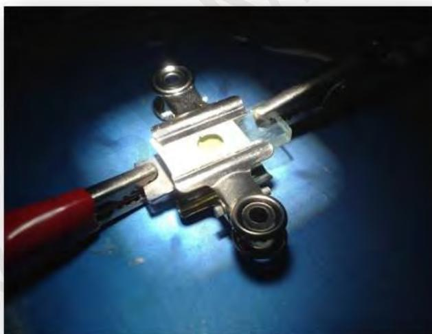
**Figure 3.2.** Image of the assembled DSSCs.
