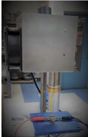
**Figure 3.3.** Solar simulator with reference cell positioned for testing.
