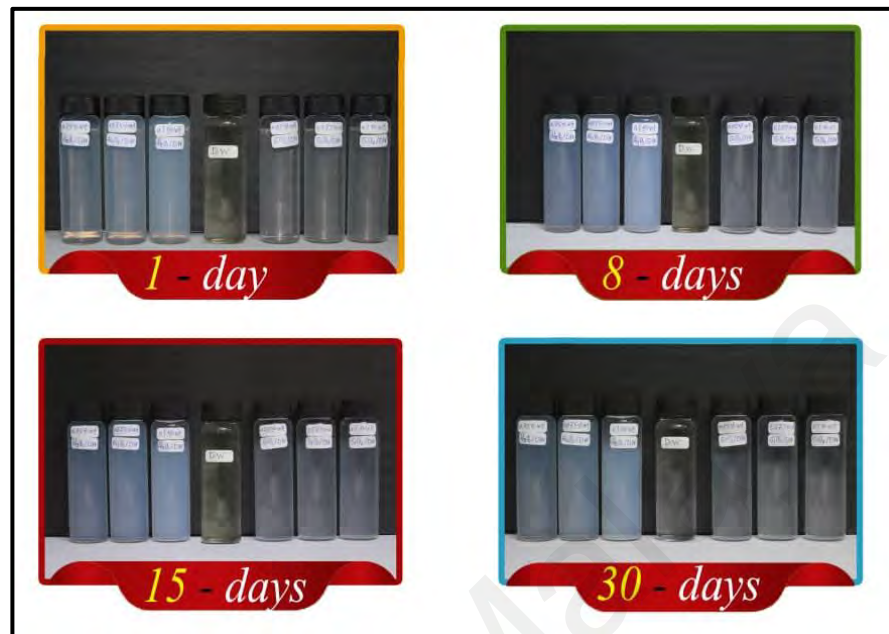
Figure 3-5: Dispersion of metal oxides nanofluids over 30 days.
