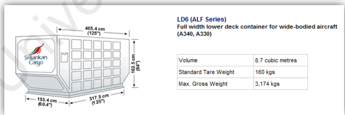
FIGURE 2.8: Dimensions of Ld6 Unit Load Devices (“ULD Container Types,” n.d)
