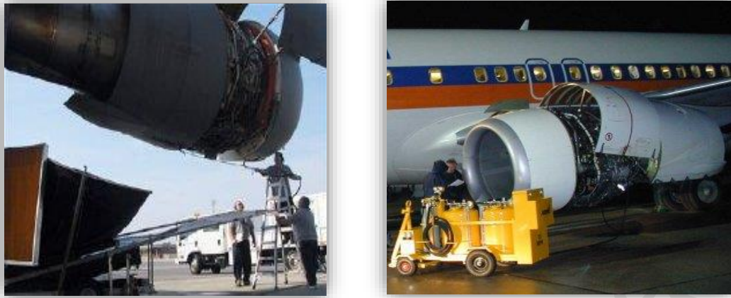
FIGURE 2.5: Engine Water Wash (AZoCleantech, 2009)
