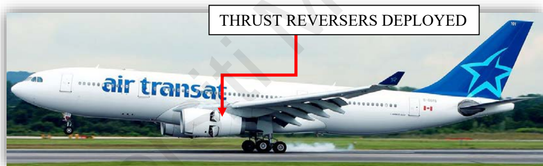
FIGURE 2.10: Thrust Reversal by Air Transat
