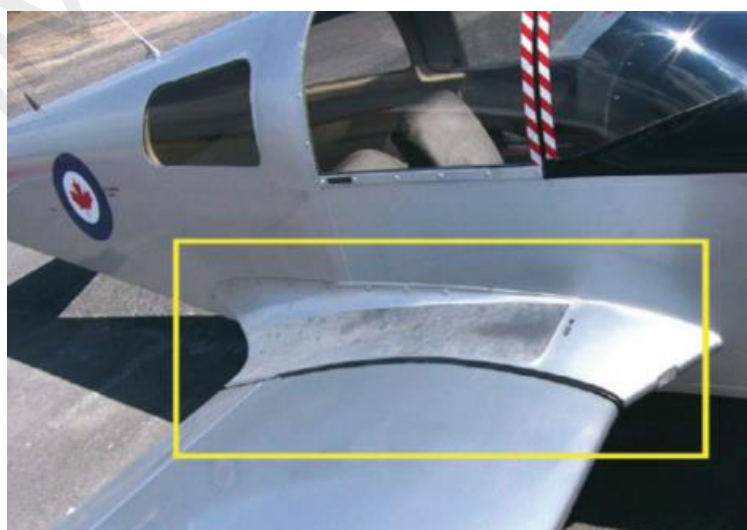
FIGURE 2.3: Interference Drag occur at wing root (Aerodynamics of Flight, February 2021)
