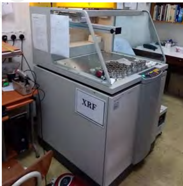
Figure 3.11: Axios XRF spectrometer
