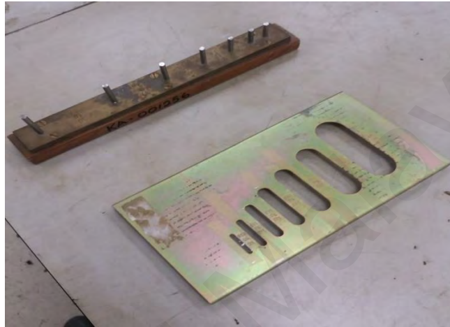
Figure 3.10: Elongation and flakiness gauges
