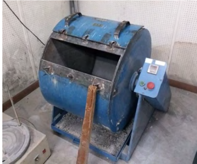
Figure 3.9: Los Angeles abrasion machine
