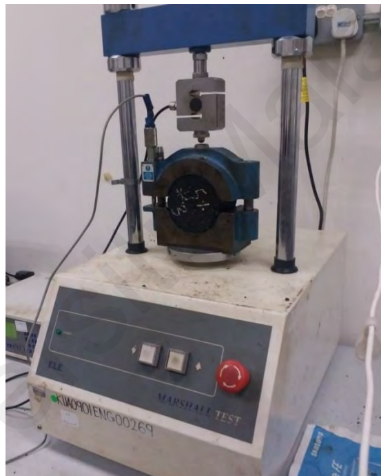
Figure 3.14: Marshall machine setup
