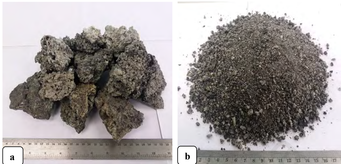
Figure 3.4: Palm oil clinker: (a) large chunks (b) crushed aggregates
