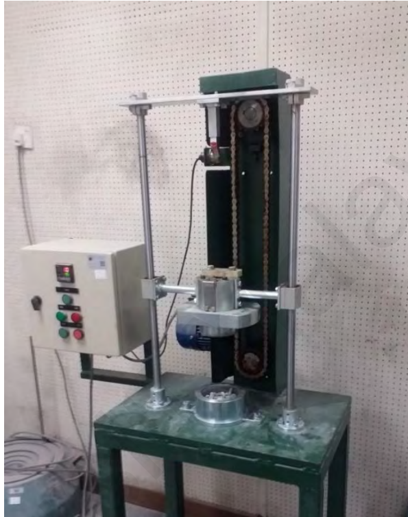
Figure 3.8: Aggregate impact test apparatus
