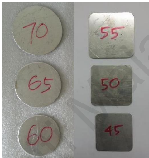
Figure 3.5: Blank samples with different sizes for circular and square sheet metal drawing
